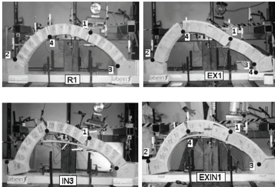
Figure 5. Failure modes and hinge position according to different strengthening lay-outs.
