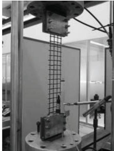
Figure 1. Pure tensile tests of four-yarn basalt textile specimen
