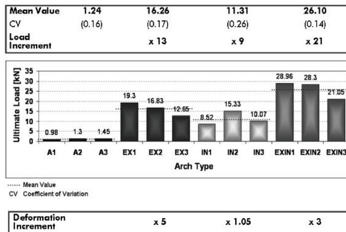
Figure 4. Results of arch testing
