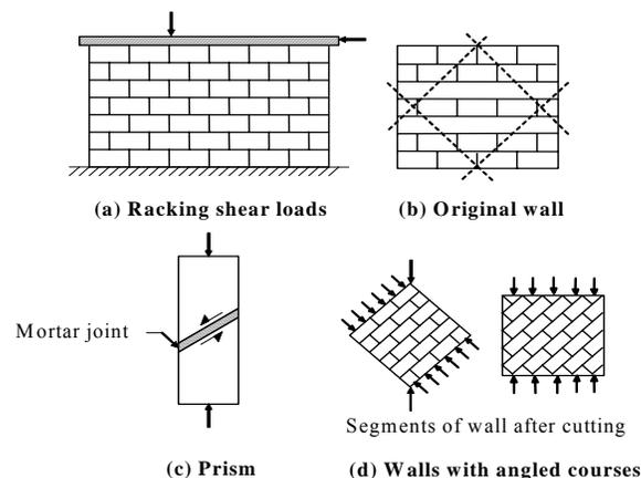
Figure 1. Test Set-up Adopted to Study Masonry Shear behaviour
