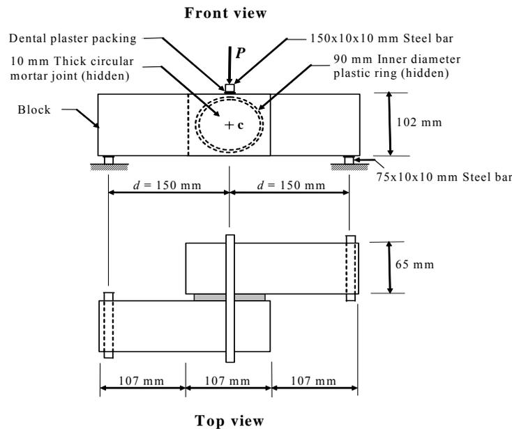
Figure 4. Load and Support Arrangements for Testing the Z-shaped Shear Specimens
