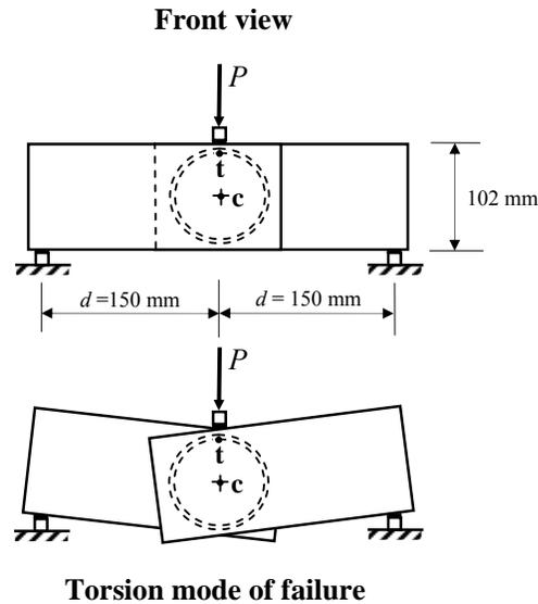
Figure 5. Observed Torsion Mode of Failure
