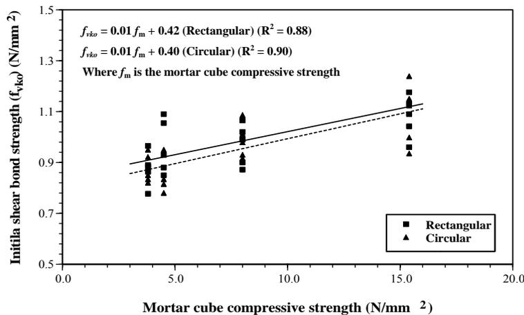
Figure 8. Initial Shear Bond Strength vs Mortar Cube Compressive Strength
