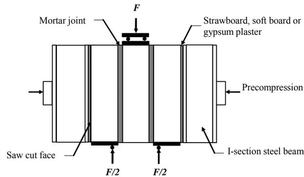
Figure 2. Triplet Test Set-up Adopted by BS EN 1052: Part 3 (2002)
