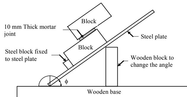
Figure 7. Apparatus Used to Determine the Coefficient of External Friction
