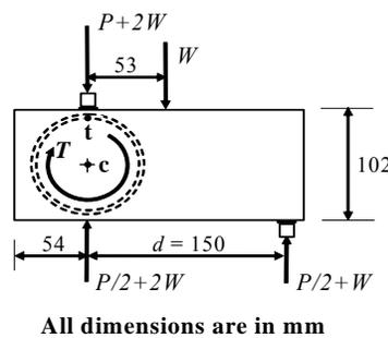
Figure 6. Free Body Diagram for Top Block
