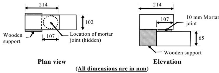
Figure 3. Example of the Method Used in Constructing the Z-shaped Shear Specimen (Circular Mortar Joint)
