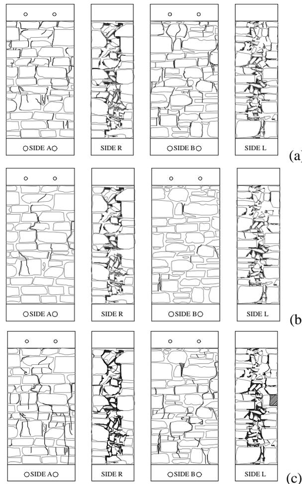
Figure 12: Cracks patterns at the same stress level before (a) and after (b) injection and after injection at the peak strength (c)
