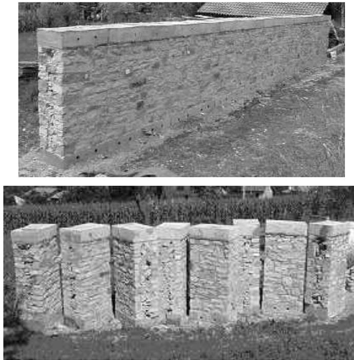
Figure 1 : View of the entire wall built and of some of the 17 specimens obtained after the wire sawing.
