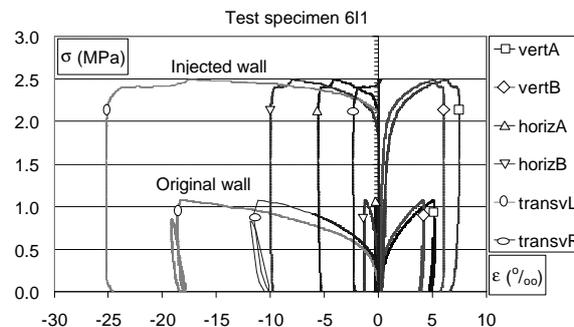
Figure 11: Stress-strain diagram after (at final strength) and before (at first loading cycle) injections.
