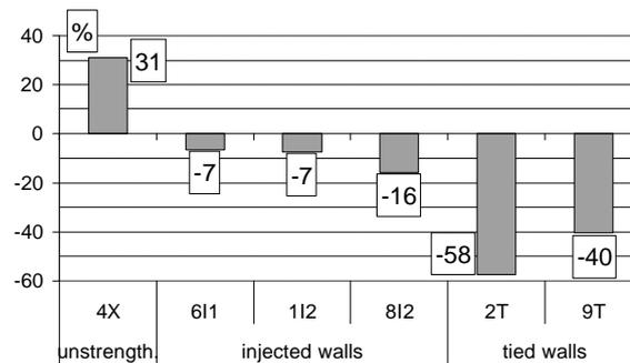
Figure 13: Transversal strain variation at the peak strength after injection and tying
