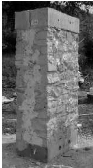
Figure 4: View of a wall before injection
