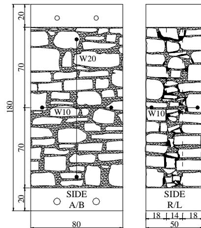
Figure 2 : Geometrical characteristics of the walls and measurement points.
