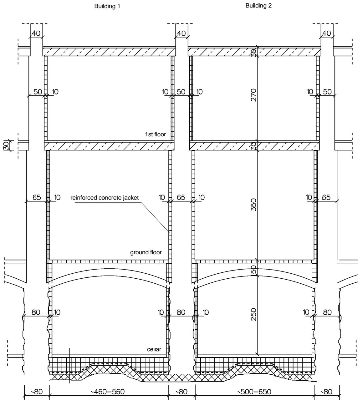
Figure 1 : Strengthening of walls by applying a reinforced concrete jacket.
