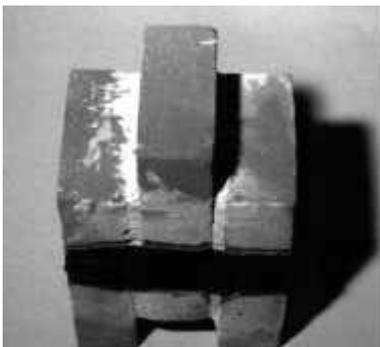
Fig. 7: Specimen after 96 Freeze/Thaw Cycles
