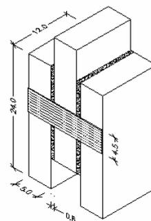
Figure 2: Reinforced specimen
