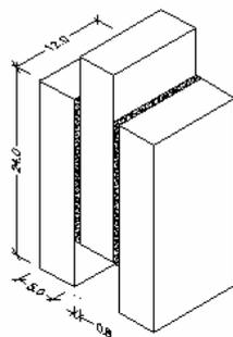
Figure 1: Unreinforced specimen
