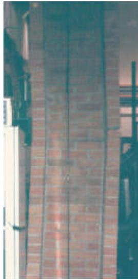
Figure 2: Cracking at “failure” in a flexure test (Sayed Ahmed et al. 1999)
