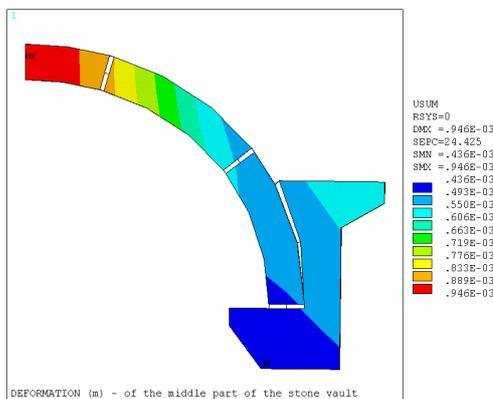
Figure 12 : Print of magnified vault distortions
