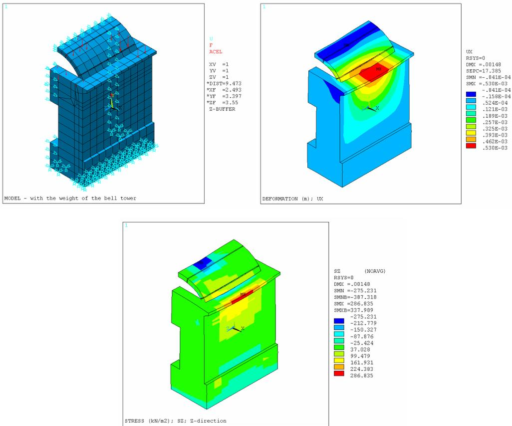
Figure 16 : Model of bearing construction with the load of the old bell tower
