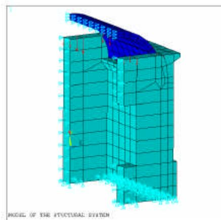
Figure 9: Three-dimensional model with gable loads
