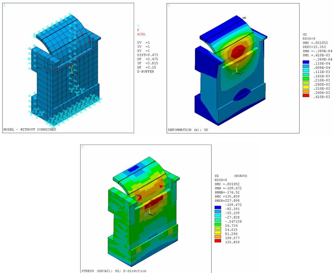
Figure 15 : Model of bearing construction without horizontal corniches
