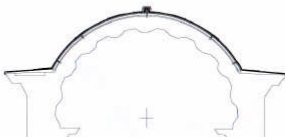
Figure 18 : Part of the cross section plan with the new lead covering
