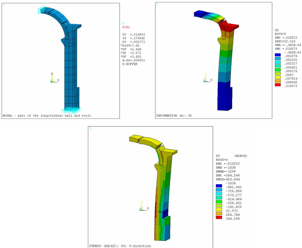
Figure 17 : Model of the part of bearing construction of the vault and longitudinal walls only
