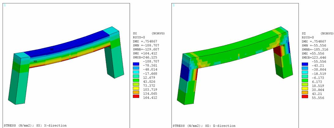
Figure 14 : Print of tension of the tie
