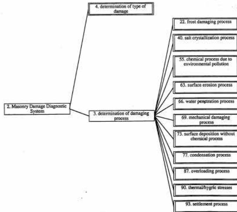
Figure 3: Decision tables tree with the damaging processes to be checked.
