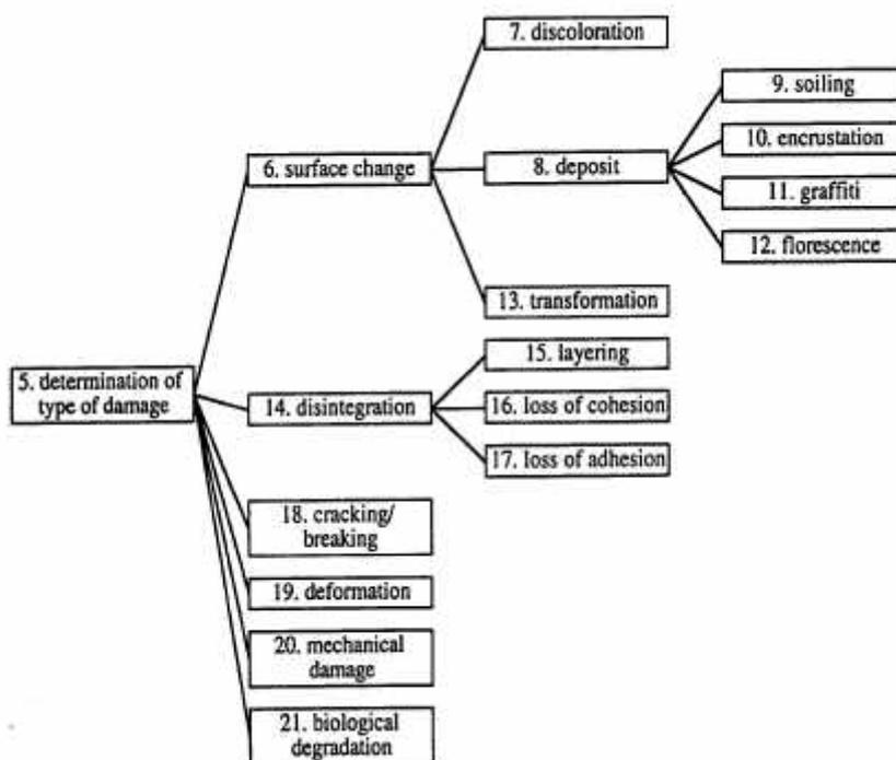
Figure 2: Decision tables tree with the different definitions of damage types, using an hierarchical approach.
