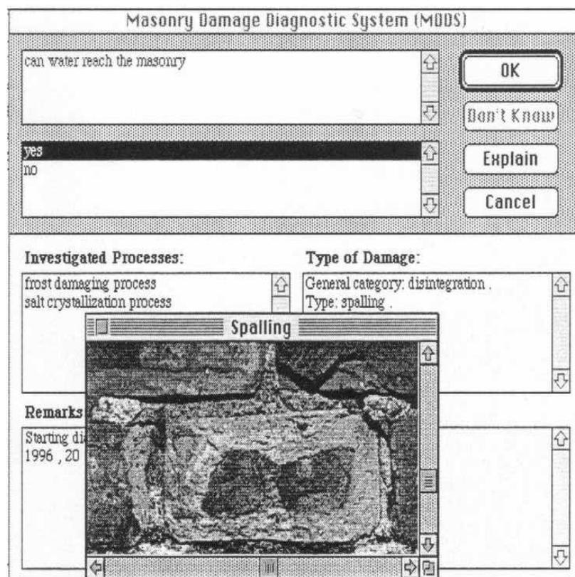
Figure 1: Typical screen picture of the first MDDS programme, showing an example of a damage type and the start of the damaging mechanism investigation.
