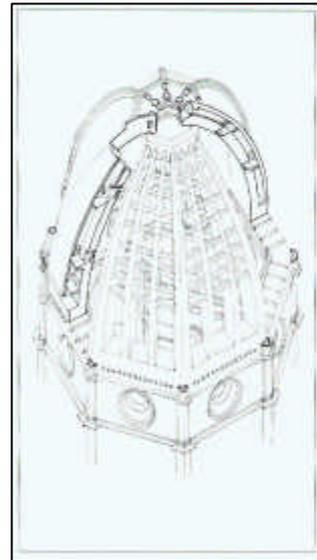
Figure 4 : Axonometry of the dome of Florence Cathedral (Murray, 1985)
