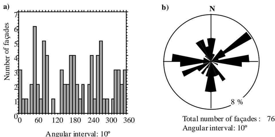
Figure 2 : Histogram (a) and rose diagram (b) of exposition azimuth of surveyed façades (given by the exposition sense of the vector normal to the façade plane).
