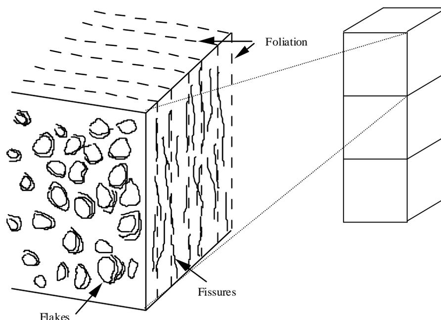
Figure 3 : Effects of foliation on fine-grained leucogranitic stones decay.
