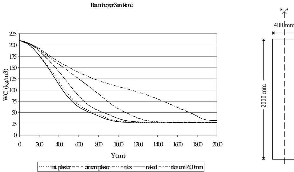
Figure 6: Comparative results of the distribution of the water content along the height of the walls, at the middle section, for baumberger sandstone
