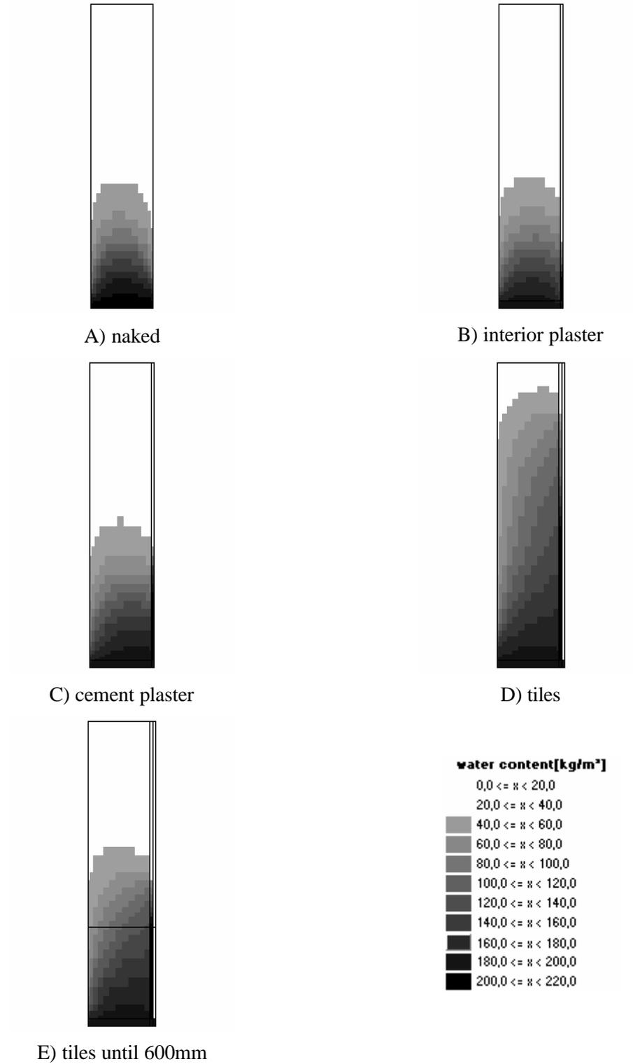
Figure 5: Distribution of the water content in the wall of baumberger sandstone after 1 year
