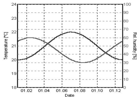
Figure 3: Interior climatic conditions approximated with sinus functions [3]
