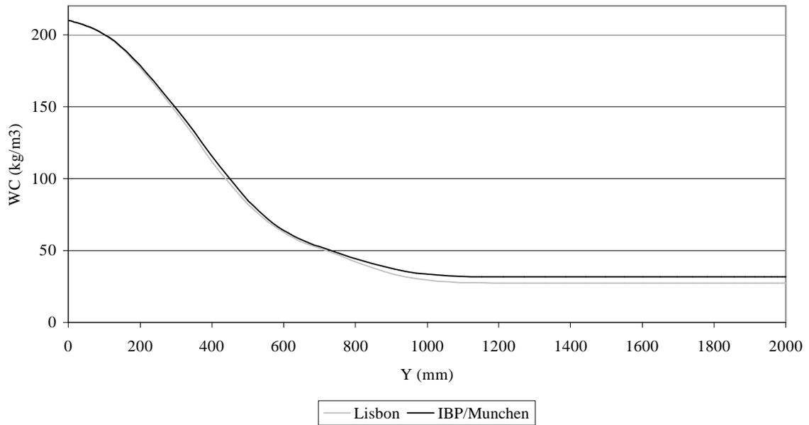
Figure 8: Comparative results of the distribution of the water content along the height of the wall, at the middle section
