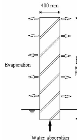
Figure 1: Schematic diagram showing the masonry stone test piece
