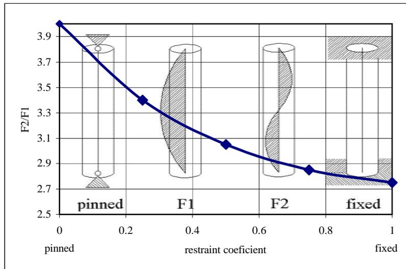
Figure 9 : Theoretical relationship between the ratio between the first and second natural frequencies ( $F2/F1$ ) and a restraint coefficient measuring the level of restraint ranging from 0 (pinned) to 1 (fixed)
