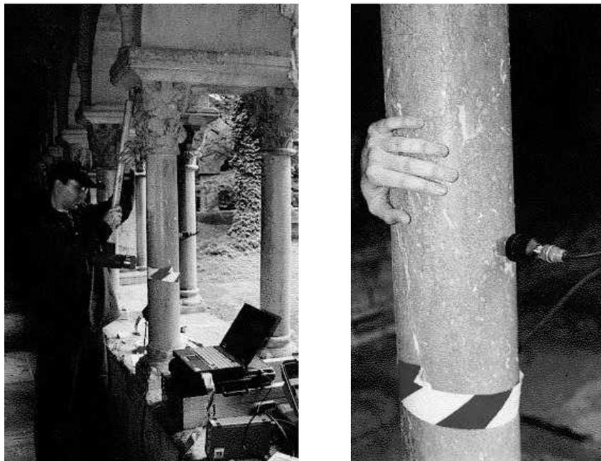
Figure 3 : Acquisition system (left) and accelerometer attached on a column (right)
