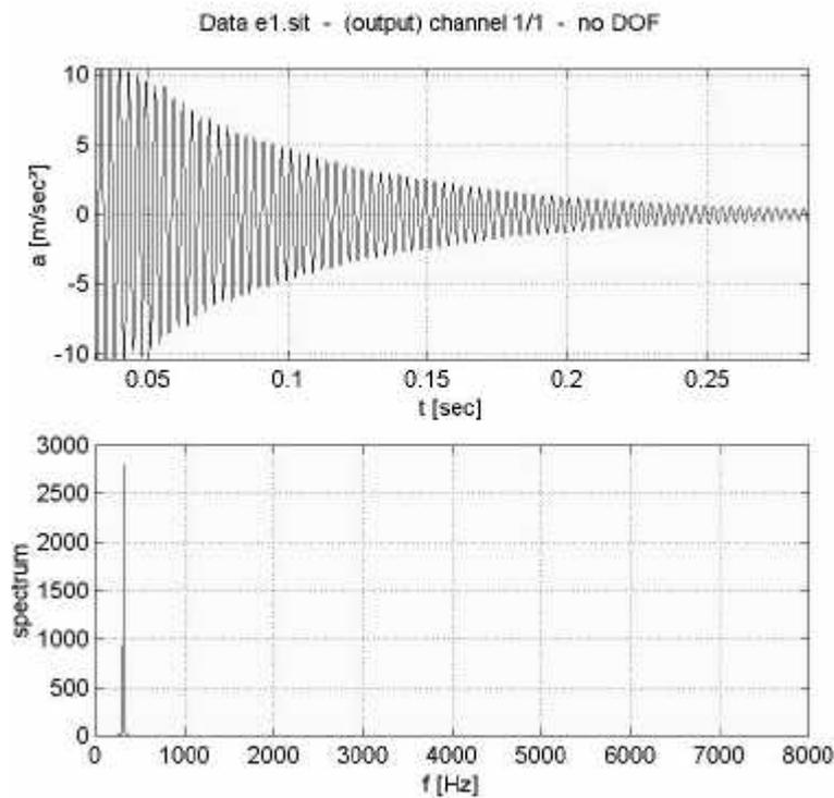
Figure 4 : Typical time-response of a column (above) and FFT diagram (below).
