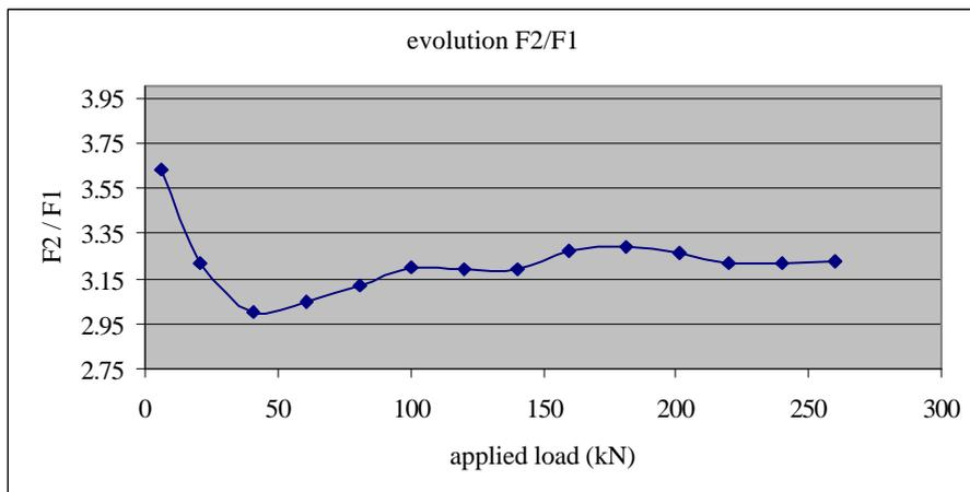
Figure 8 : Relationship between the ratio F2/F1 and the applied axial load.
