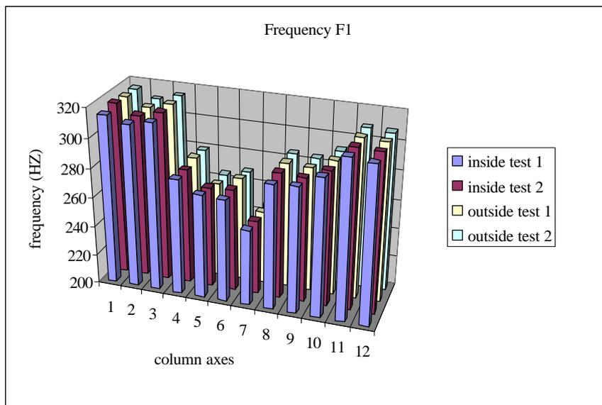
Figure 5 : Distribution of first frequency in the cloister columns (1 to 12).
