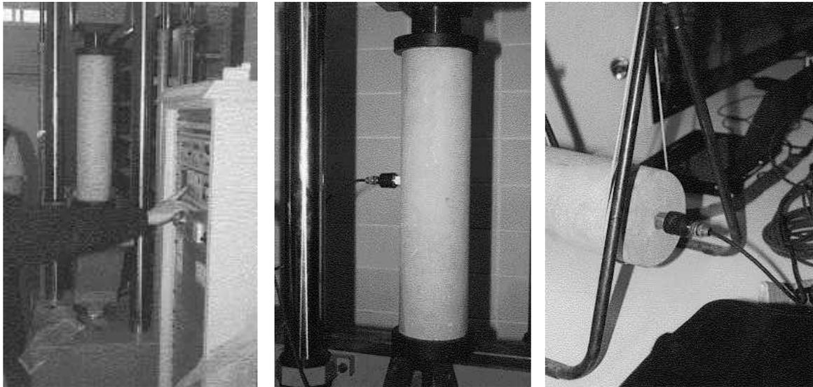
Figure 6 : Detail of test (left), attached accelerometer (middle) and dynamic modulus test (right)
