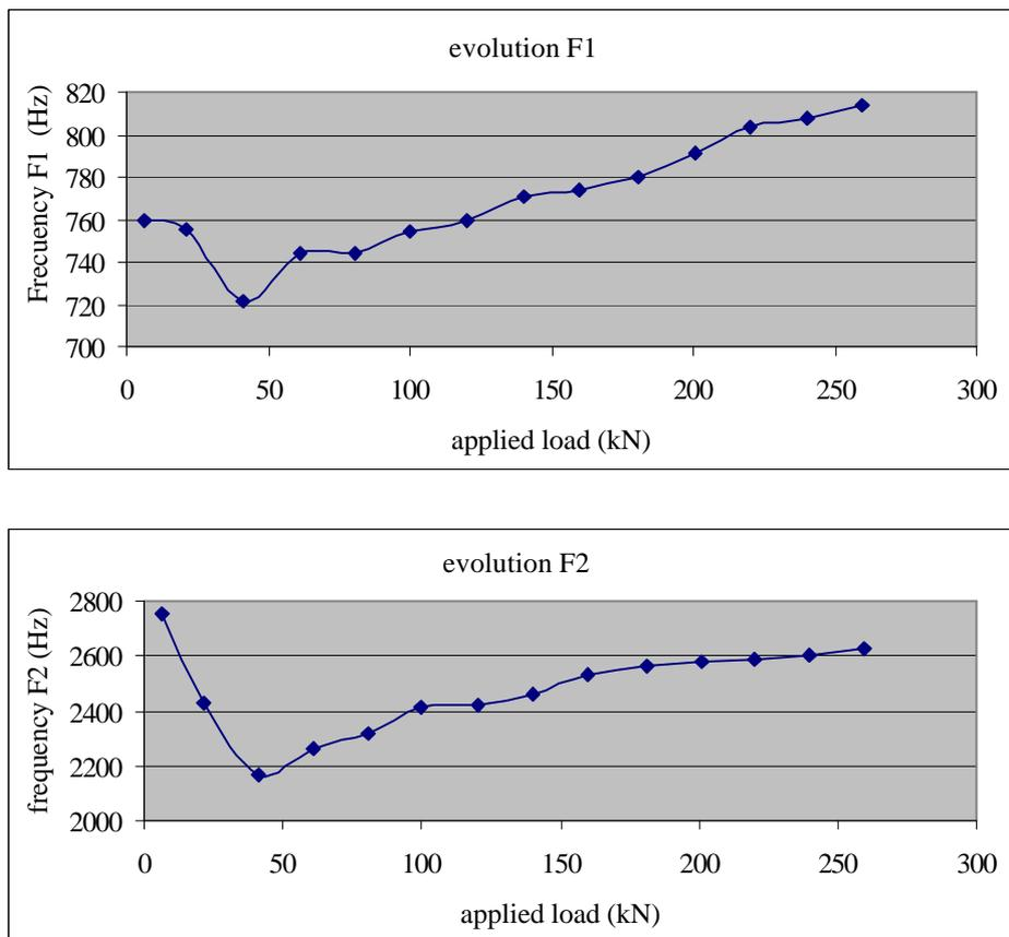
Figure 7 : Evolution of the natural frequencies with the applied axial load. First frequency (above) and second frequency (below).
