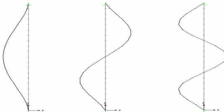
Figure 9. First modes of vibration predicted by the analytical model, corresponding to frequencies  $F1=370$  Hz (left);  $F2=909$  Hz (middle);  $F3=1700$  Hz (right).
