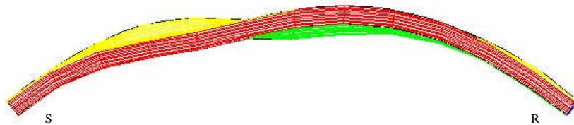
Figure 13 Deformed shape of skew arch calculated with ANSYS
