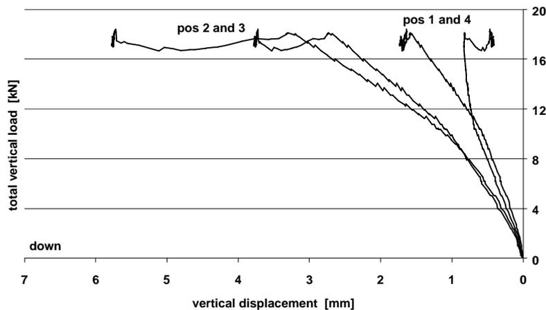
Figure 8 Vertical displacements versus the total of the four equal loads (down is positive).
