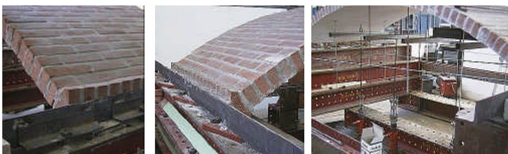
Figure 6 Details of the supports and load introduction
