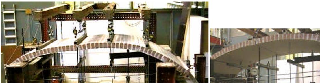
Figure 10 Deformed arch almost at the end of testing, and crack beneath largest load, position 2, test R1
