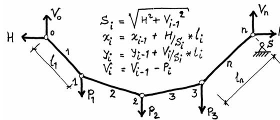
Figure 3 Finding the shape of a string with weights by calculation
