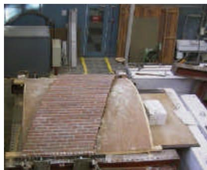
Figure 4 A skew arch resting on its formwork.
