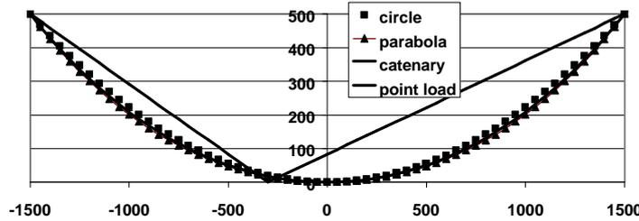
Figure 1 The shape of a catenary compared with circle segment and parabola
