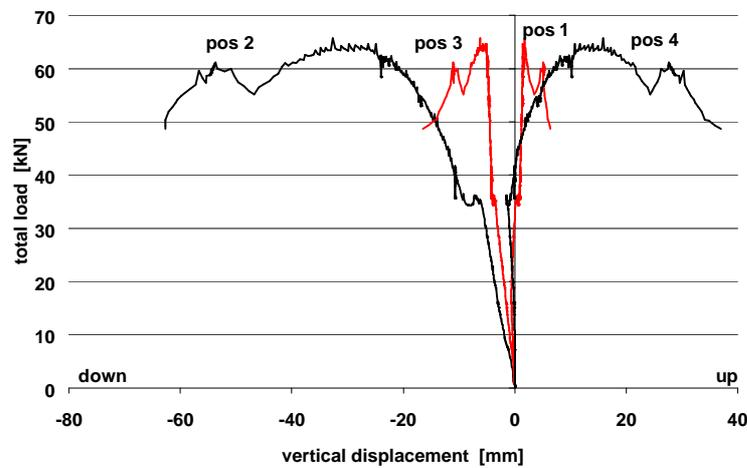
Figure 9 Vertical displacements versus the total of three equal and one larger load.
