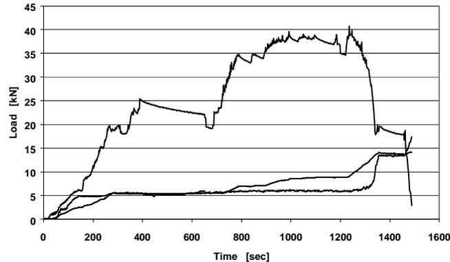
Figure 7 Load versus time for test R1, final load cycle
