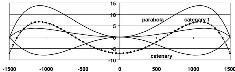
Figure 2 Differences (in mm) between catenary, parabola and circle segment
