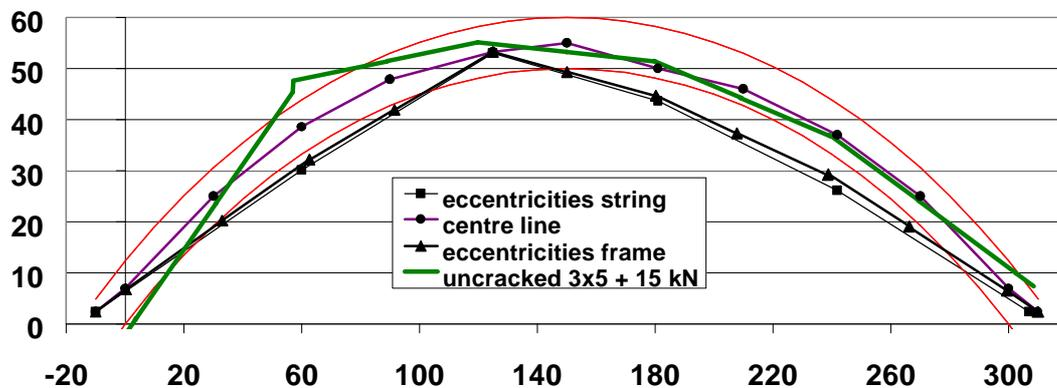
Figure 12 Eccentricities (or thrust line) in the three pinned arch
