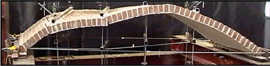
Figure 11 collapse of skew arch S2
