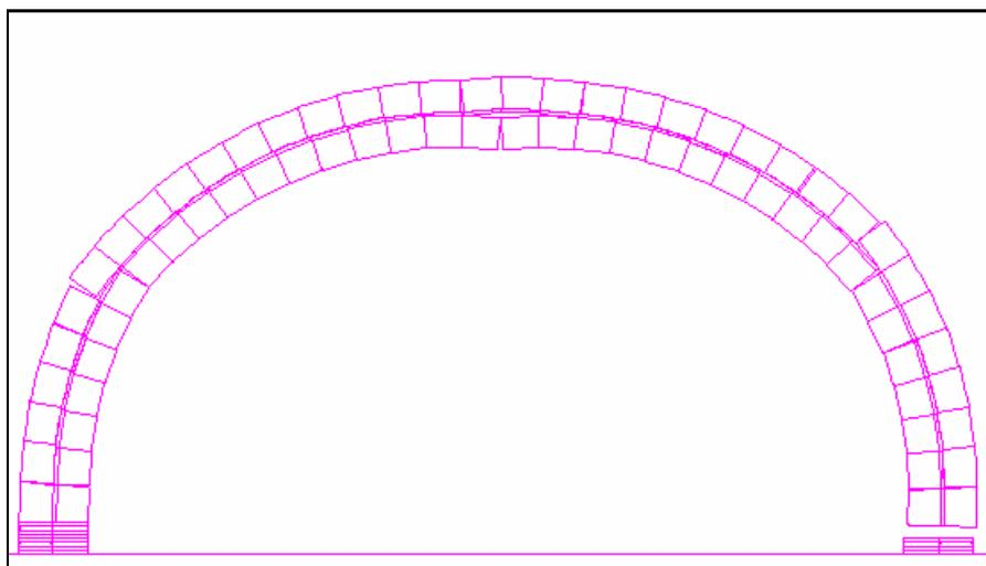
Figure 9 : Beginning of collapse due to arch base horizontal displacement and rotation
