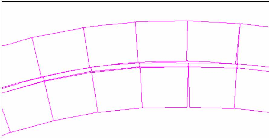
Figure 8 : Separation of layers at the keystone due to base rotation
