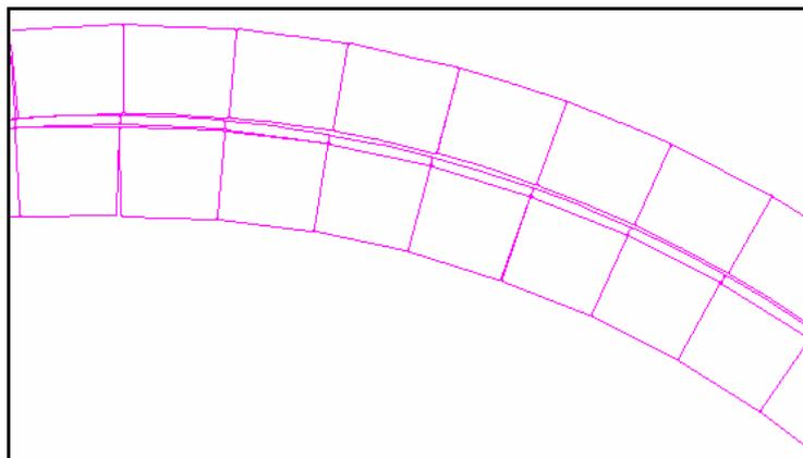
Figure 5 : Separation between the arch layers
