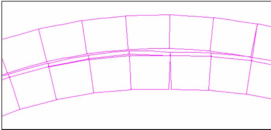
Figure 7 : Separation between the arch layers near to the keystone, due to base rotation
