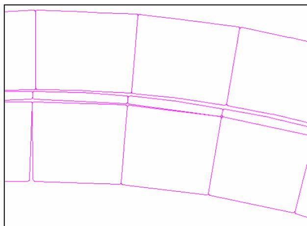
Figure 6 : Separation between the arch layers close to the keystone
