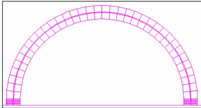
Figure 4 : Block assemblage of the multiple-leaf arch
