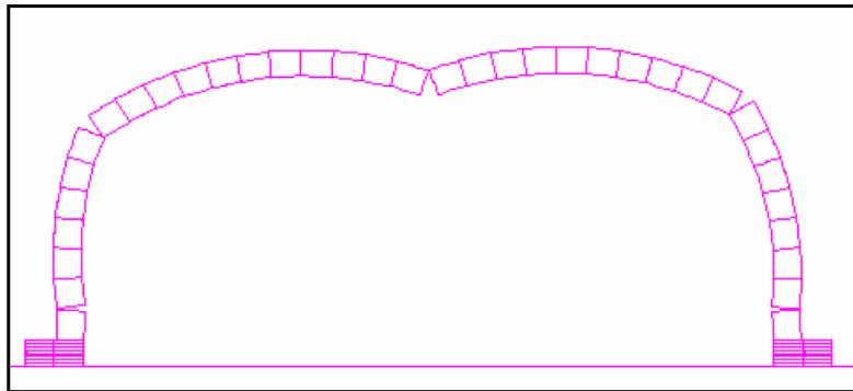
Figure 1 : Collapse of the stone masonry arch.
