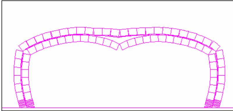
Figure 2 : Collapse of multiple-leaf arch with weak joint
