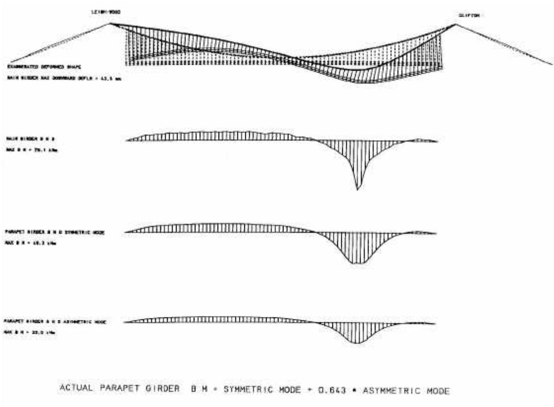
Figure 4: A4 Tonnes vehicle in one lane at quarter span.
