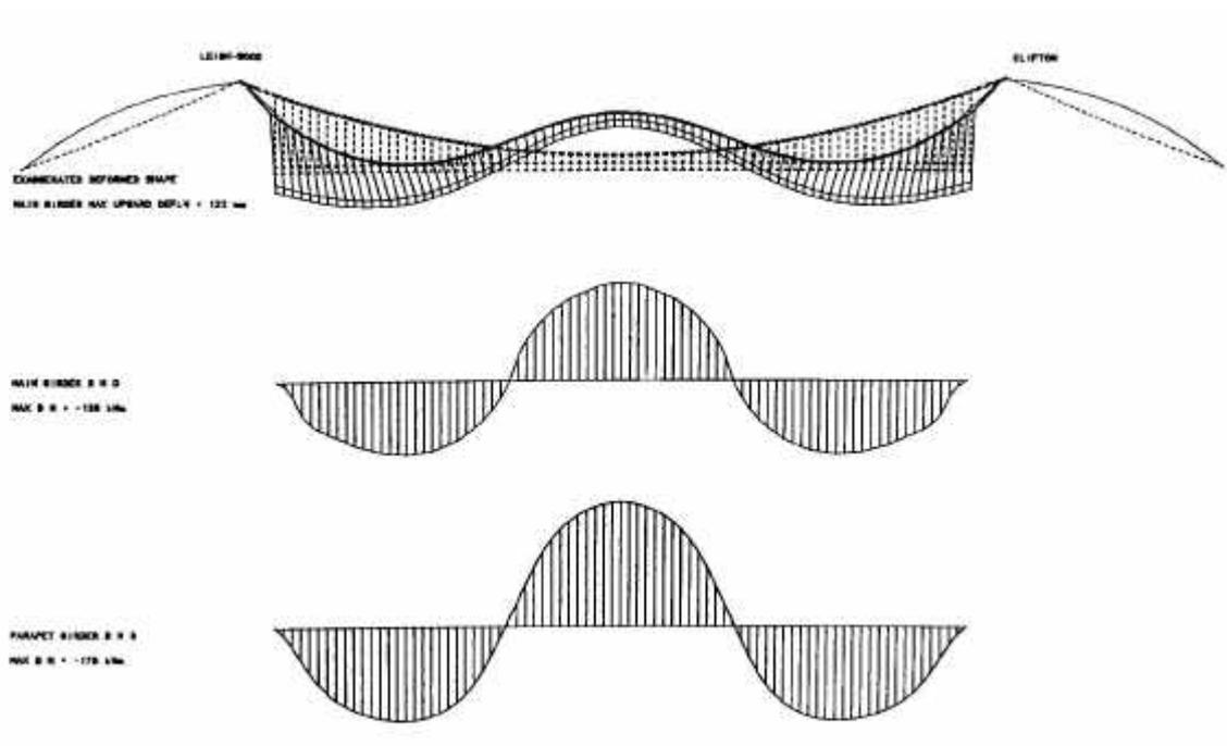
Figure 3 : Both lanes at the ends of the span loaded with UDL.
