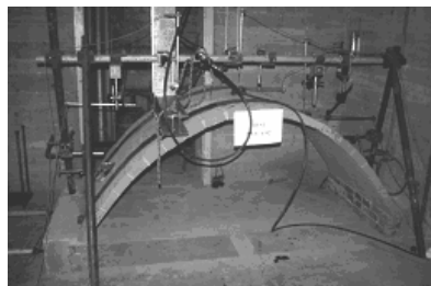
Figure 6 : Experimental set-up and position of the transducers.
