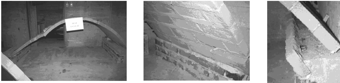
Figure 7 : Shear sliding along a mortar joint: final global deformation and details of the failure in the first joint closest to the springer (EX.C.01 and EX.G samples).
