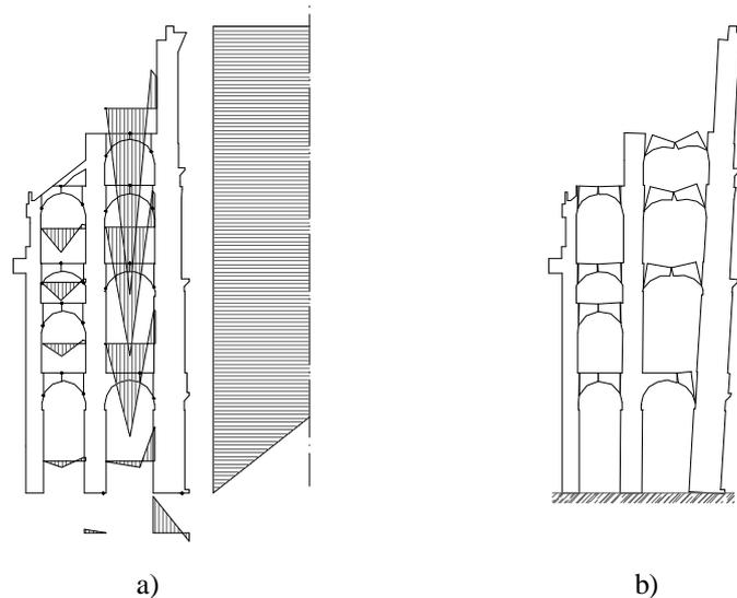
Figure 9: a) vertical and horizontal displacements; b) radial section of the mechanism.
