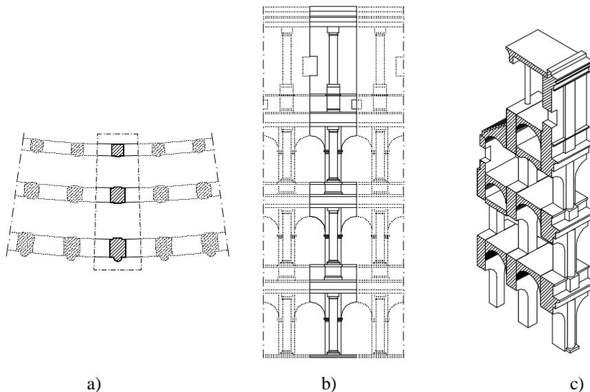
Figure 3: Module of the structure: a) plan; b) front view; c) axonometry.
