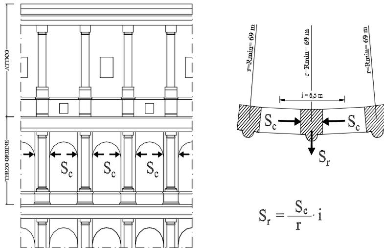
Figure 11: Radial components of the thrusts.
