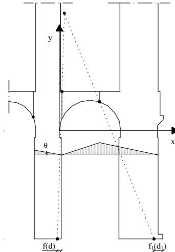
Figure 8: Rotation centres and vertical displacements related to the first level vault.
