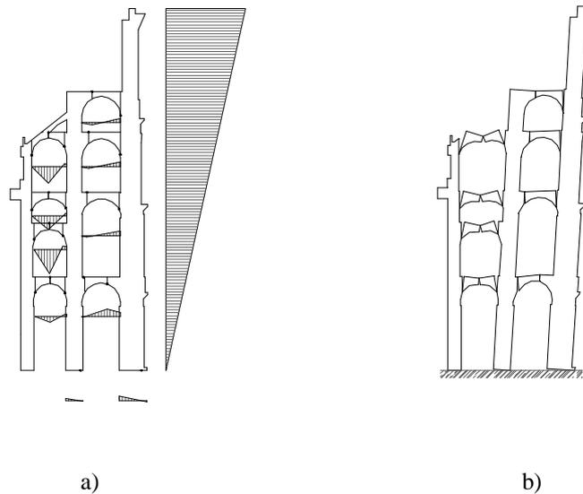
Figure 7: a) vertical and horizontal displacements; b) radial section of the mechanism.
