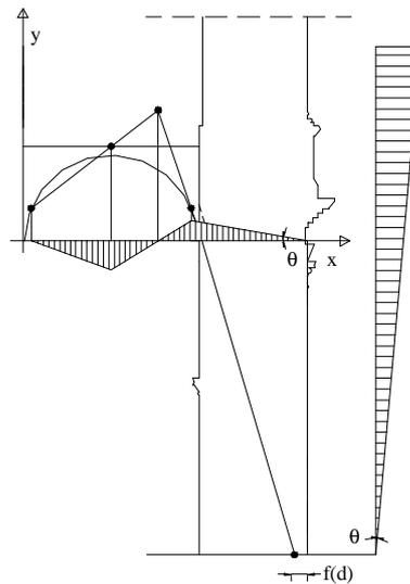
Figure 5: Rotation centres and displacement field related to the first level internal vault.
