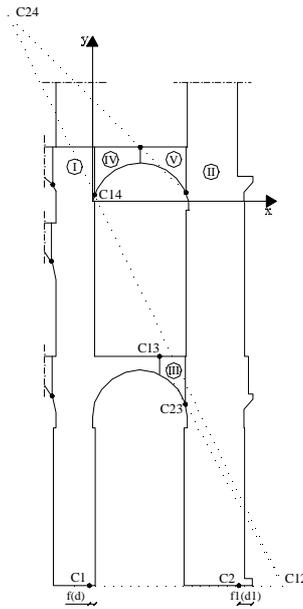
Figure 10: Rotation centres and vertical displacements related to the first level vault.
