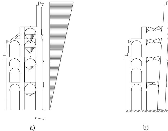
Figure 4: a) vertical and horizontal displacements; b) radial section of the mechanism.
