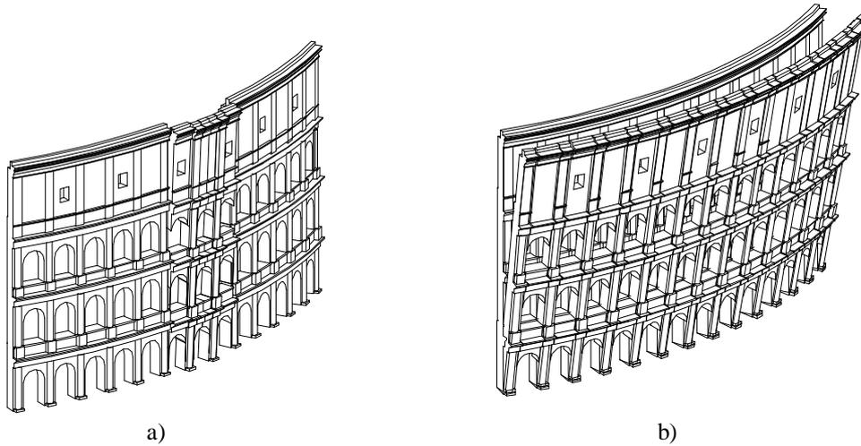
Figure 2: The external wall: a) the incompatible mechanism; b) the compatible mechanism.
