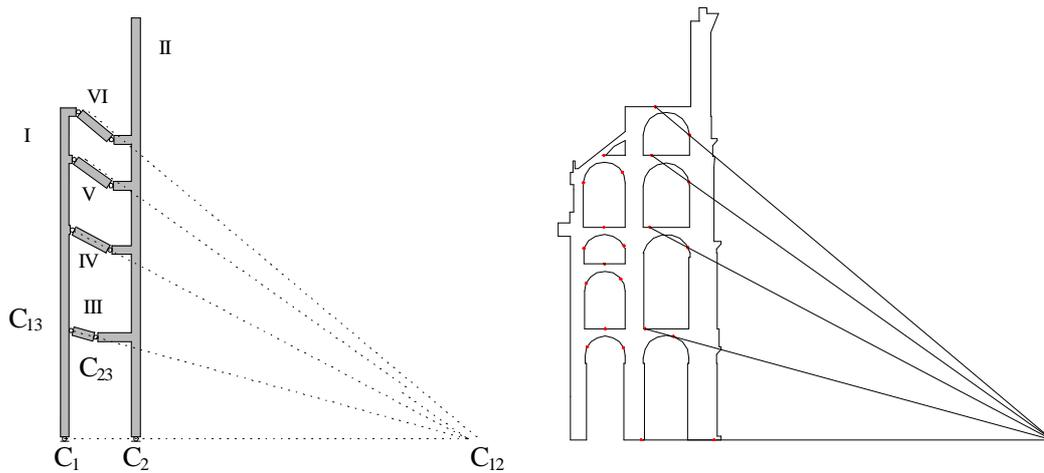
Figure 6: The alignment of the rotation centres to make the structure become a mechanism.
