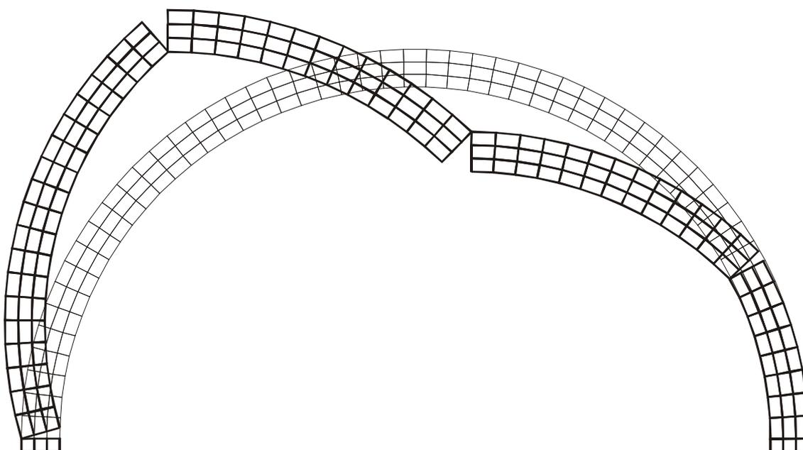
Figure 3 : Case II - Deformed mesh corresponding to a total load of 1770kN and a maximum displacement of 183mm beneath load line (displacements magnified 5 times)
