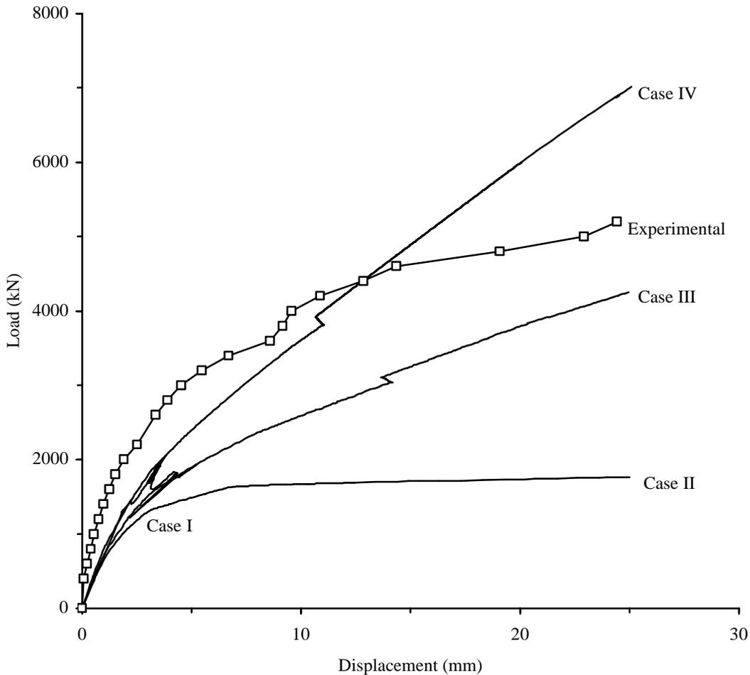
Figure 2 : Vertical displacement of arch soffit beneath load line
