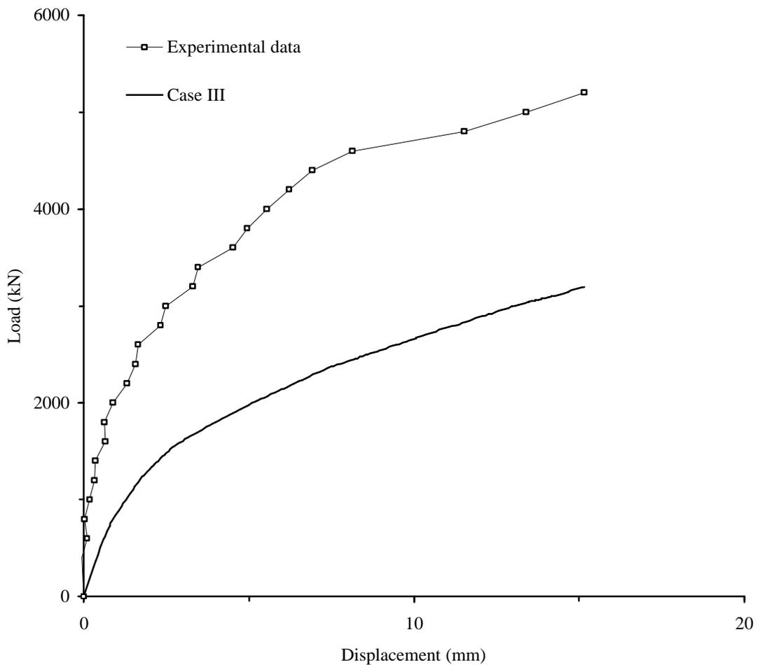
Figure 4 : Case III - Horizontal displacement of arch soffit at crown
