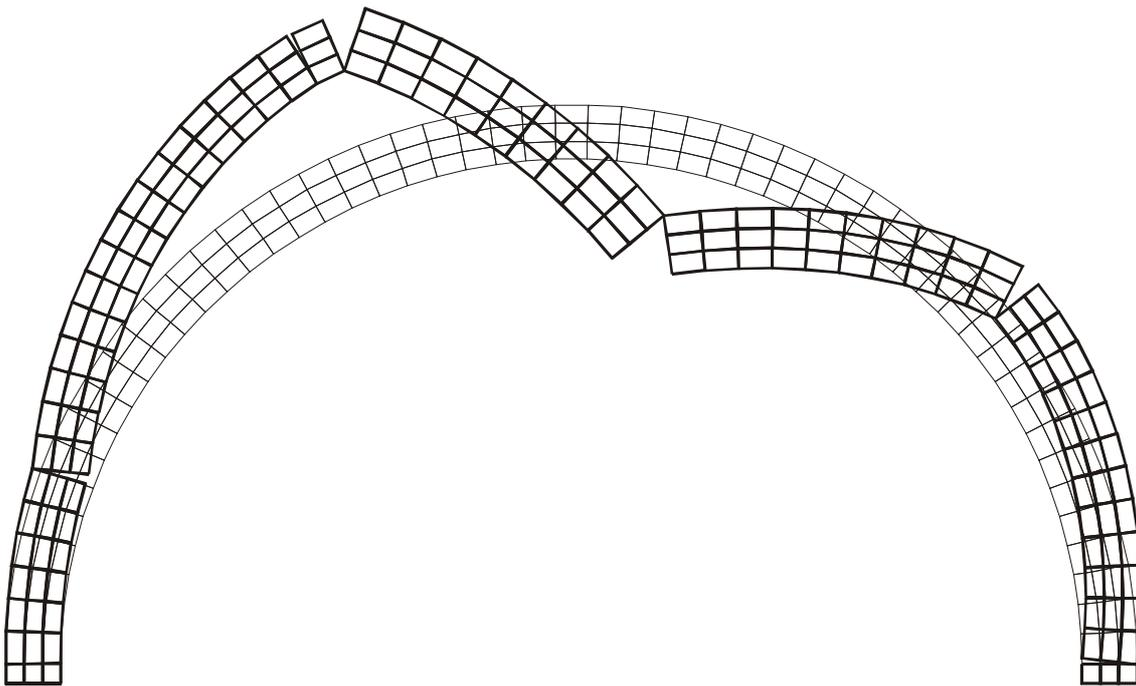
Figure 5 : Case III - Deformed mesh correspondent to a total load of 8150kN and a maximum displacement of 79mm beneath load line (displacements magnified 10 times)
