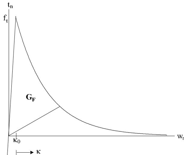
Figure 1. Exponential softening relationship adopted in the damage model
