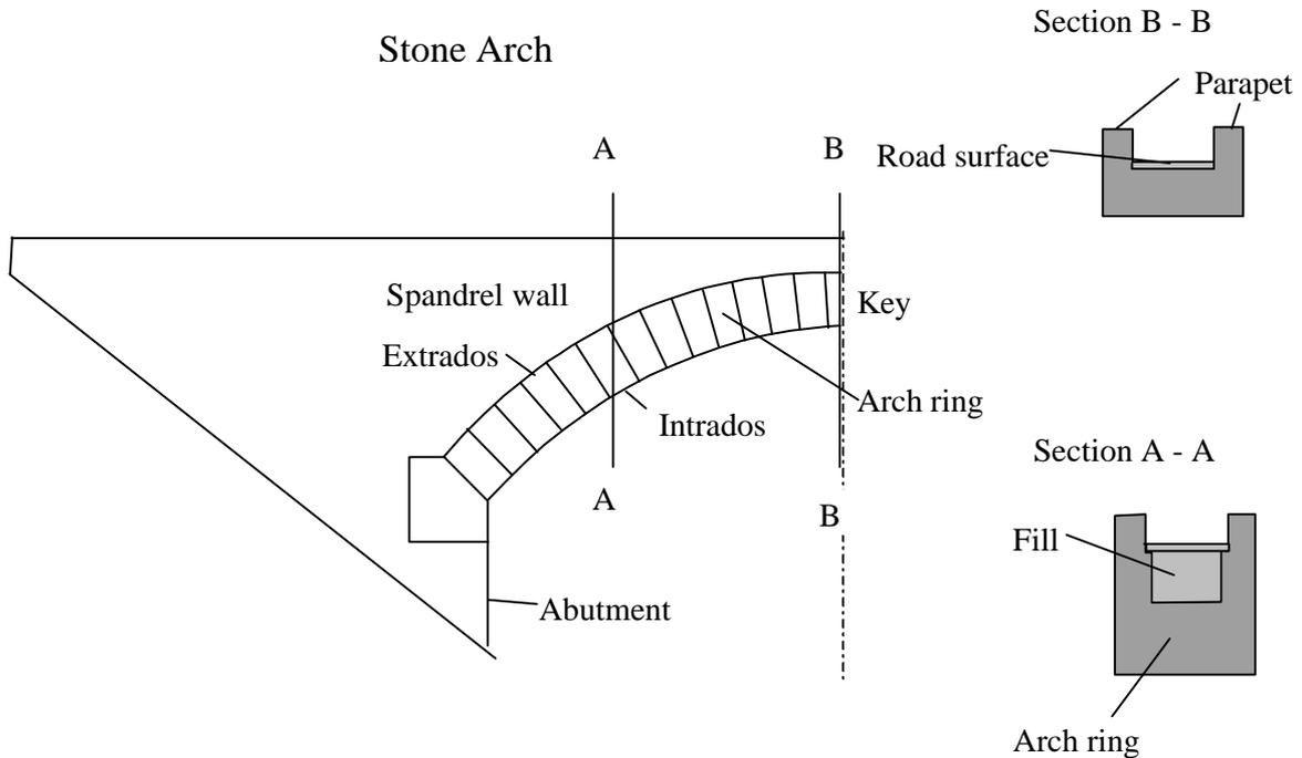
Figure 1 : Typical stone arch bridge (Porta) construction
