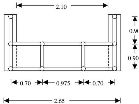
Figure 2 : Plane frame idealisation of the cross-section at the arch key of the Porta bridge
