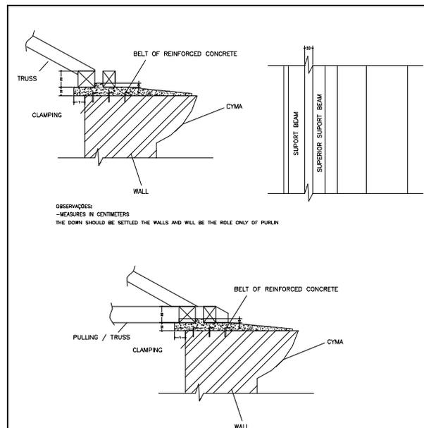
Figure 6 – Detail Showing the contact between the truss and the wall plate.
