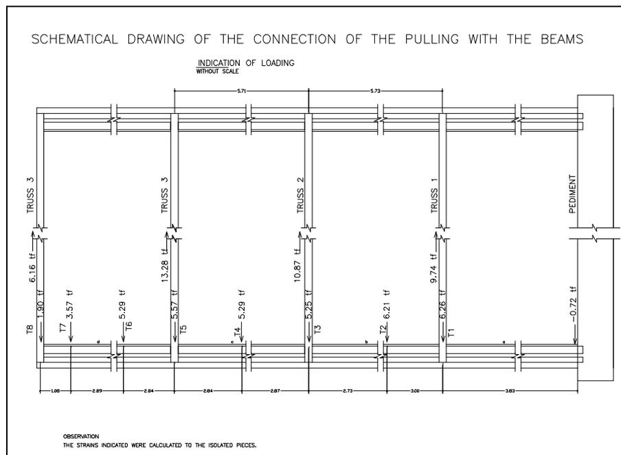
Figure 4 - Connections in Pieces from the Truss.
