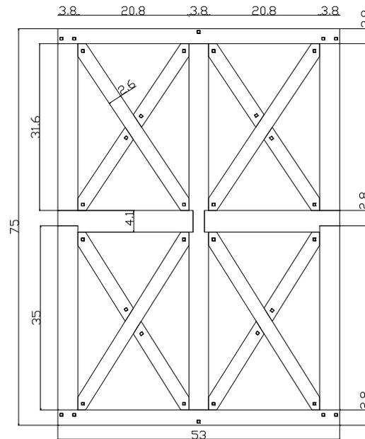
Figure 1 : Dimensions of wall panel timber frame elements (cm)
