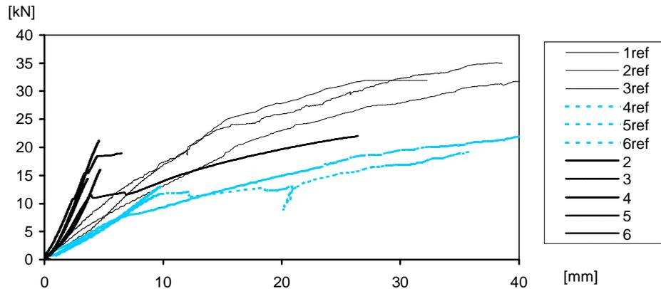
Figure 10 : Load-displacement diagrams obtained in diagonal compression of the wall panels, prior to and after strengthening (for deformation up to 40mm only)
