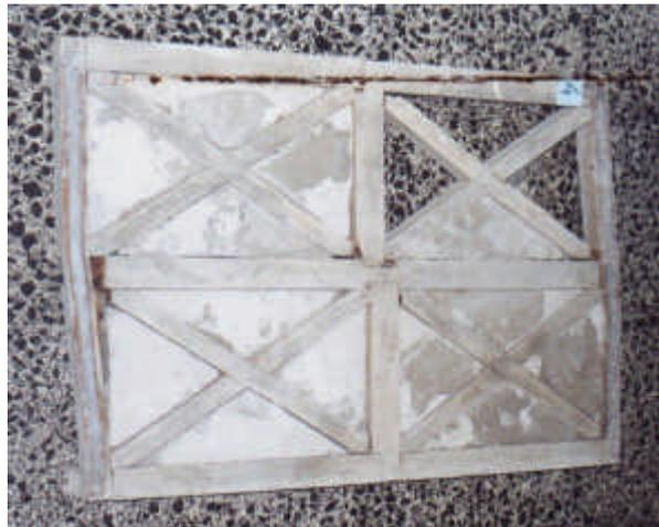
Figure 8 : Strengthened wall panel after diagonal compression test (typical failure)
