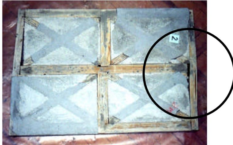
Figure 4 : Detail of the timber member failure in bending
