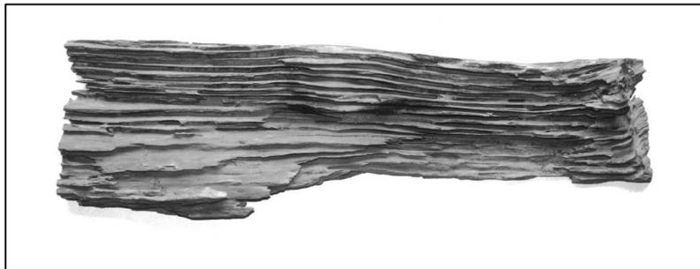
Figure 1: Aspect of typical termite damage to wood
