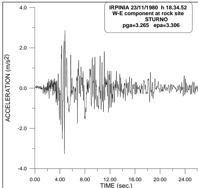
Figure 5: Irpinia Earthquake, WE component accelerogram recorded at Sturmo
