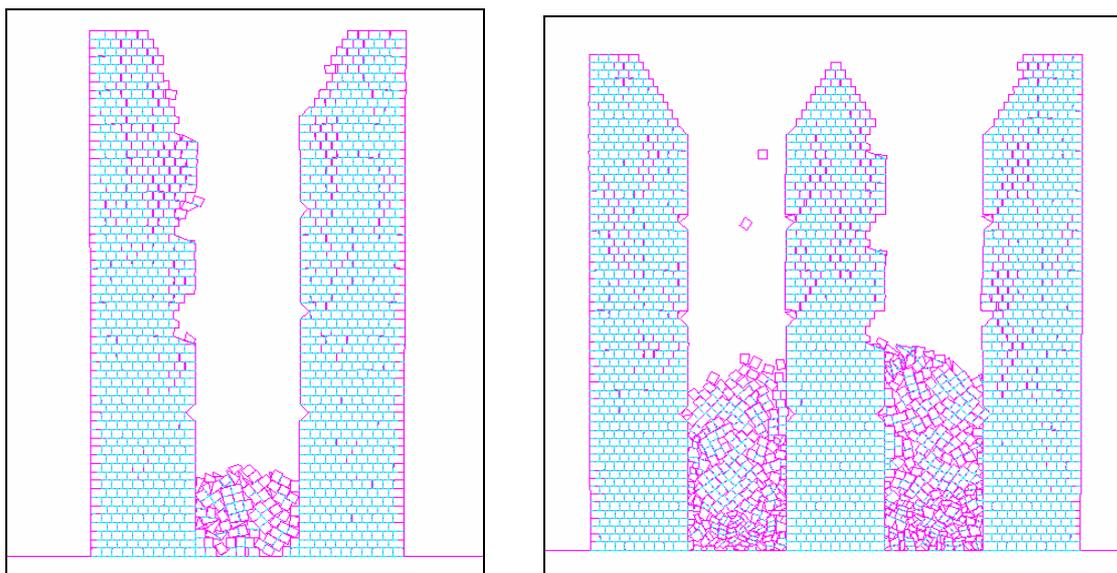
Figures 9 - 10: Aqueduct pillars with small initial damages; Sturmo Record
