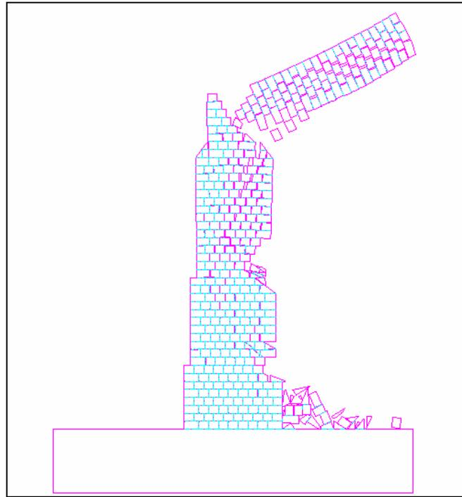
Figure 13 : Transverse failure process at 15 seconds; Sturmo record
