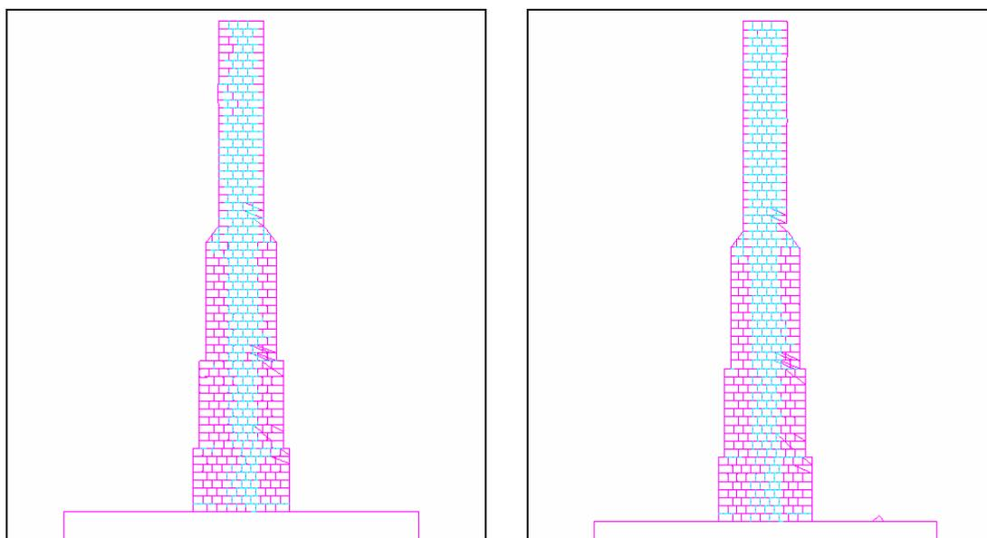
Figures 11 - 12: Transverse loading, seismic action Type 1
