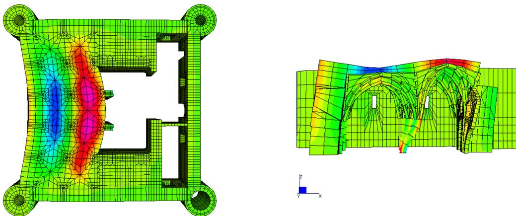
Figure 4: First vibration mode of the structure ( $f_1=5.4$  Hz)
