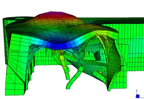
Figure 5: 4th mode of the structure (10.44Hz; section).
