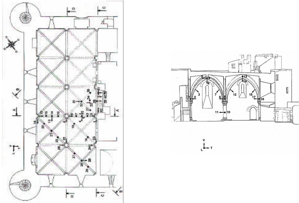
Figure 2: Excitation and measure positions of dynamic tests.
