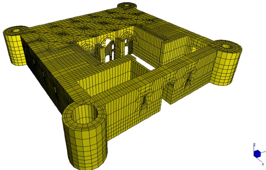
Figure 3: Finite element model of the castle
