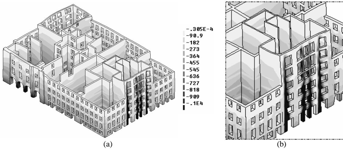
Figure 6: Compressive stresses for vertical loading (kPa): (a) complete block; (b) detail of reinforced concrete columns.
