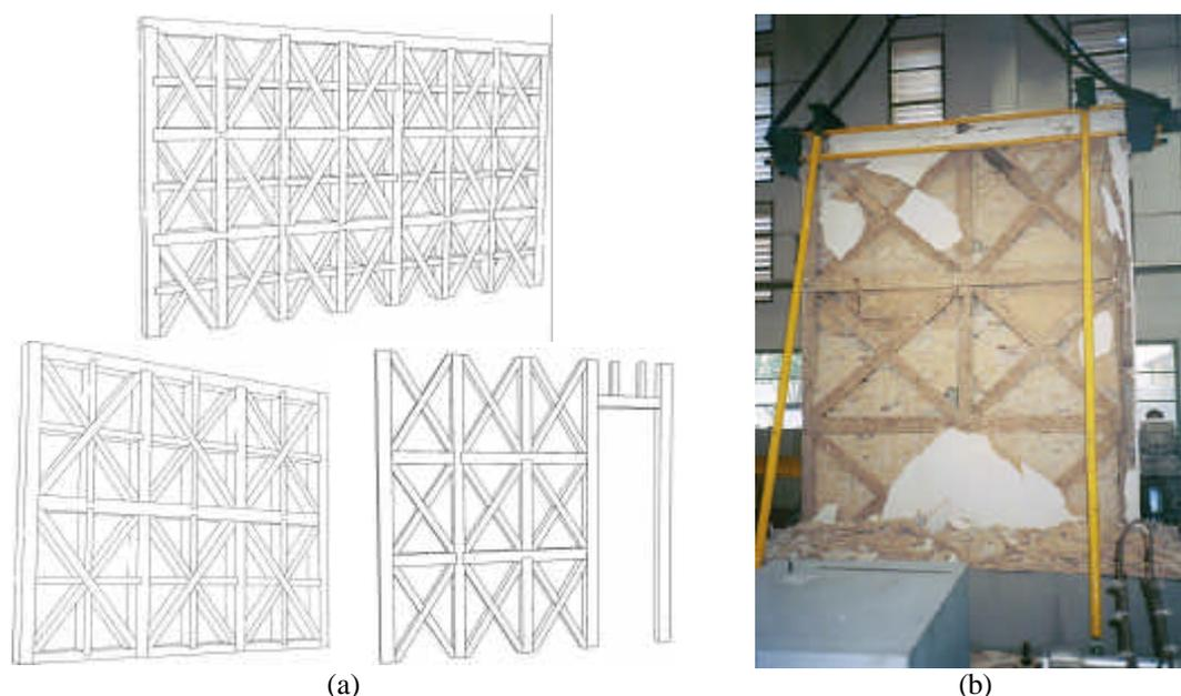
Figure 3: Examples of the composite timber-masonry walls: (a) three main types of internal timber arrangement; (b) a large specimen recovered from a demolition, used for laboratory test up to collapse.
