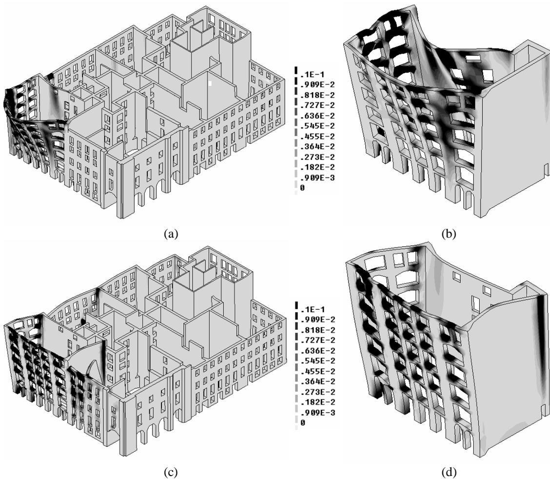
Figure 7: Cracking in the model at ultimate load for a horizontal load combination (maximum principal strain): loading in the x direction for (a) block (safety factor is 0.7) and (b) single building (safety factor is 0.7) and loading in the z direction for (c) block (safety factor is 0.7) and (d) single building (safety factor is 0.5).
