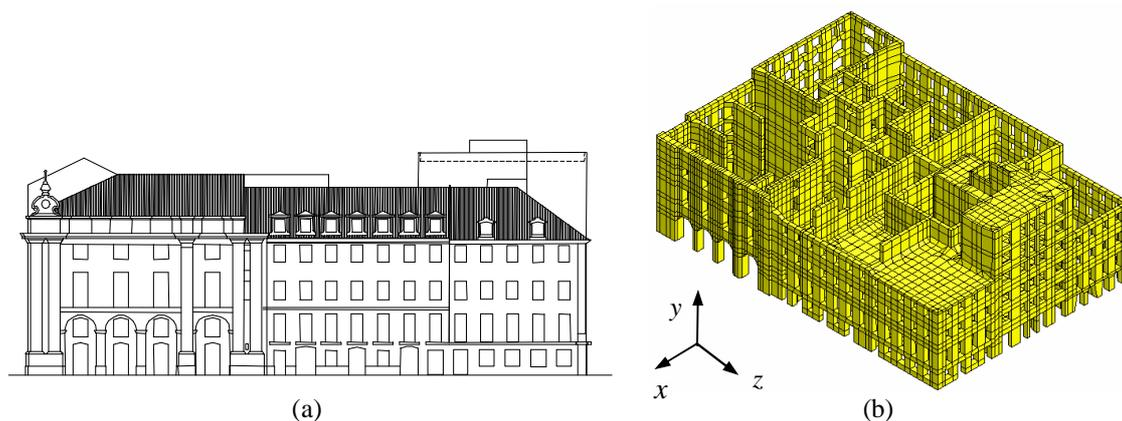
Figure 5: Case study for “block effect” analysis: (a) main view; (b) adopted finite element mesh.
