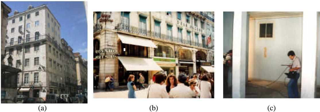
Figure 4: Main changes in Lisbon’s historical downtown buildings: (a) extra floors; (b) opening enlargement and wall removal; (c) addition of reinforced concrete and steel members.
