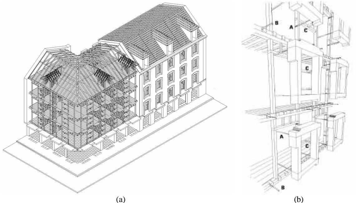
Figure 2: Aspects of the Pombaline construction: (a) building with the façade walls removed to show the timber bracing system; (b) detail of the timber frame and anchoring system to the main façade pilasters.
