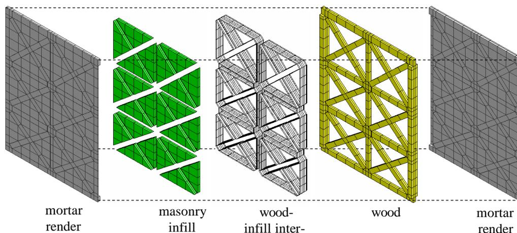
Figure 8 : Detailed model of a timber framed panel (3365 elements).
