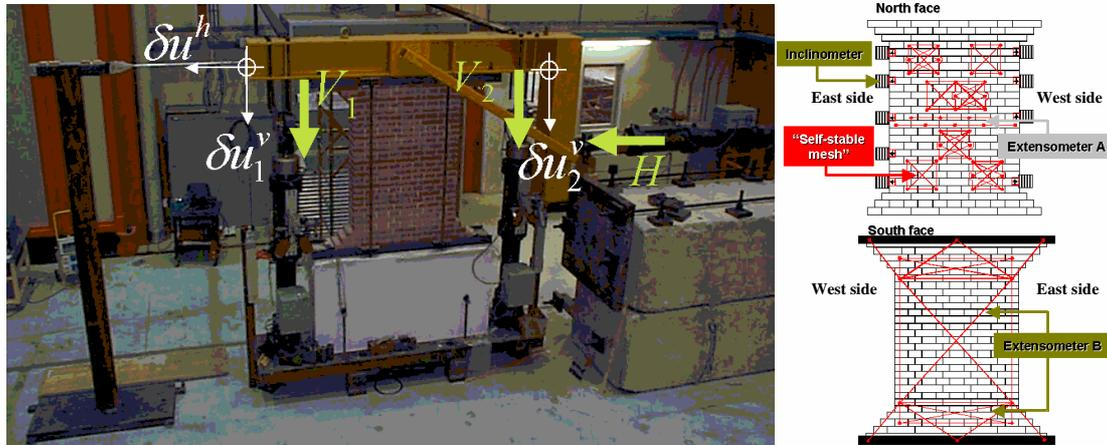
Figure 2: Test setup and instrumentation for the wall.
