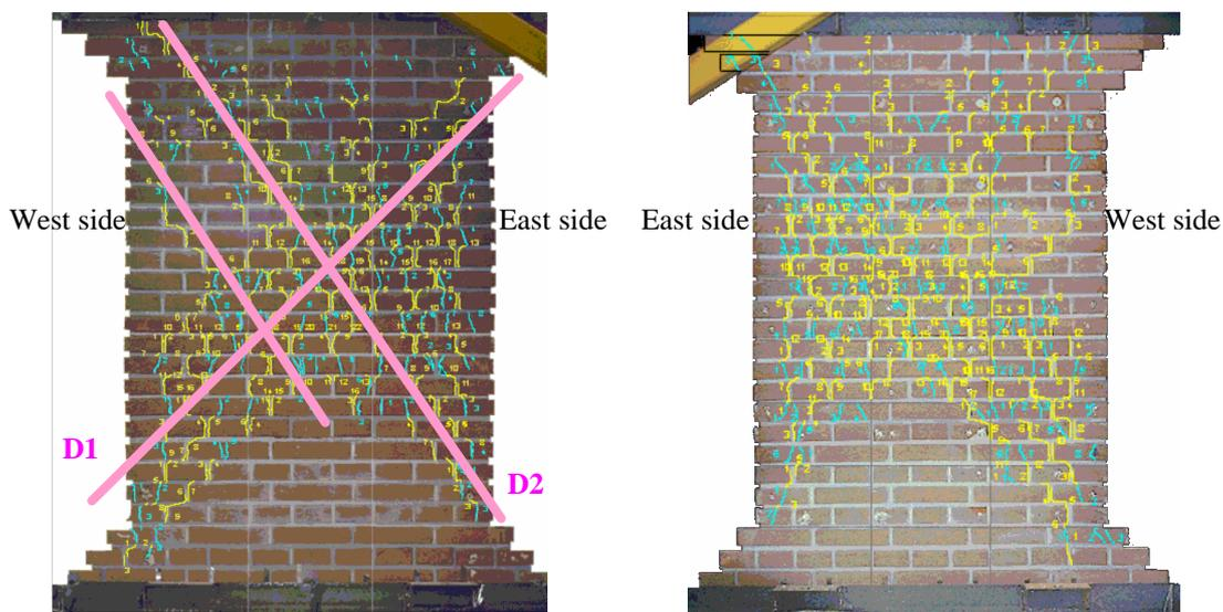
Figure 6: South (left) and north (right) crack pattern.
