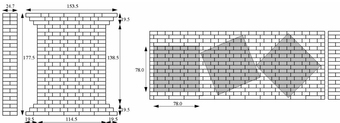
Figure 1: Dimension of the shear walls and of the wallettes.
