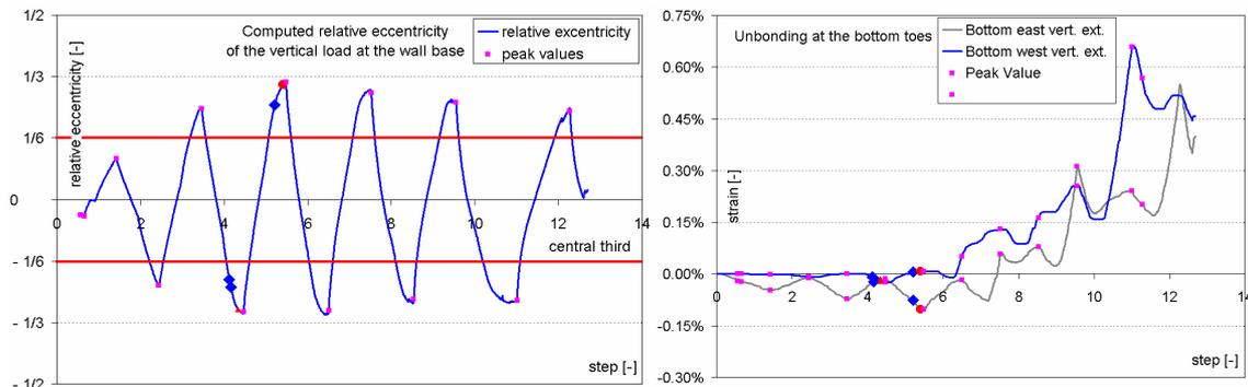
Figure 4: Relative eccentricity and toes unbonding strains versus load step.
