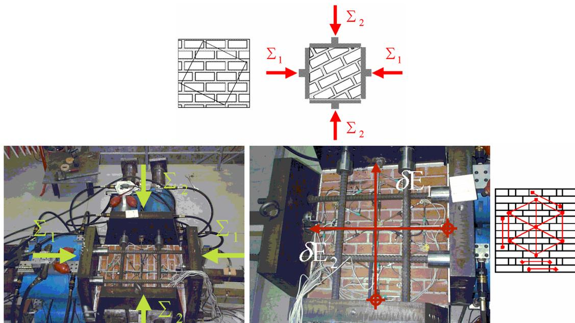
Figure 8: Test principle, setup and instrumentation for the wallette.
