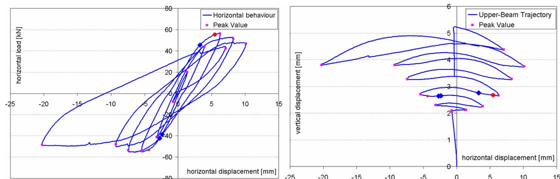
Figure 3: Horizontal load and vertical contraction versus horizontal displacement.
