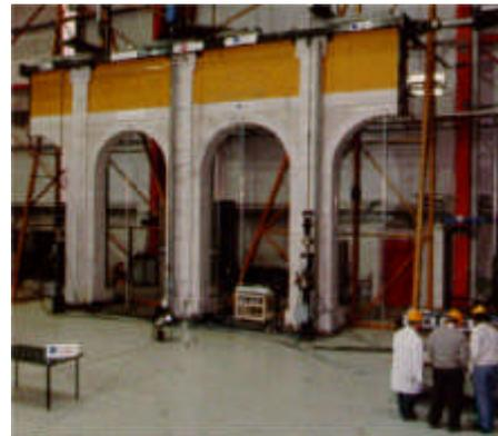
Figure 6: Façade full-scale model in the ELSA reaction wall laboratory
