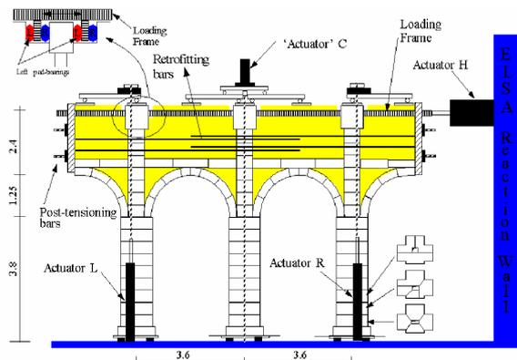
Figure 5: S. Vicente de Fora: model - Test set-up (schematic)
