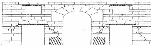
Figure 2: Cracking pattern observed after test N-200
