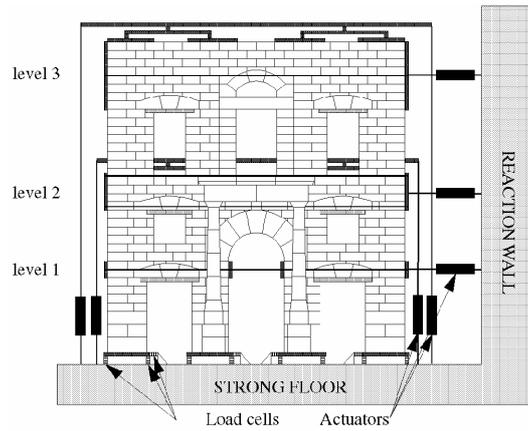
Figure 1: Test Model and loading system
