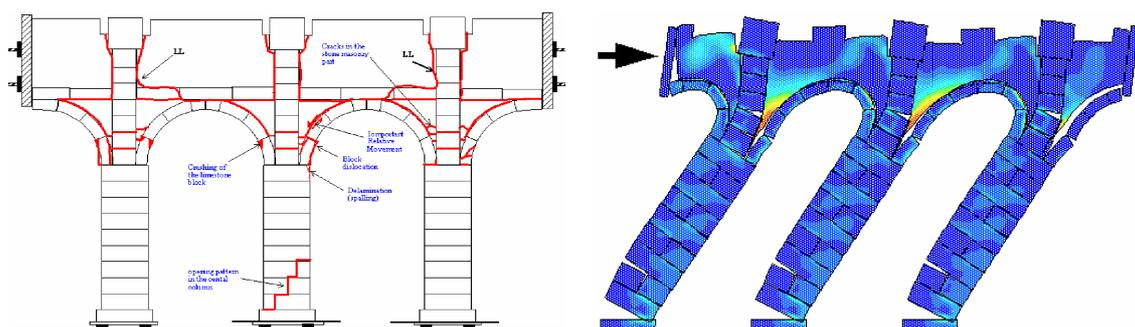
Figure 7: Damage and Deformation: a) Damage from tests, b) Deformation pattern (analytical results)
