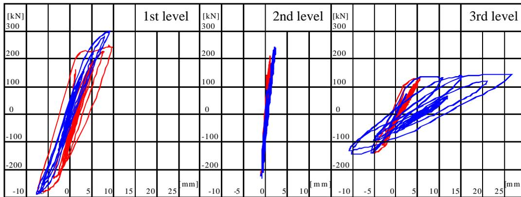
Figure 4: Interstorey shear-displacement curves during tests N-200 (grey) and R-200 (black)
