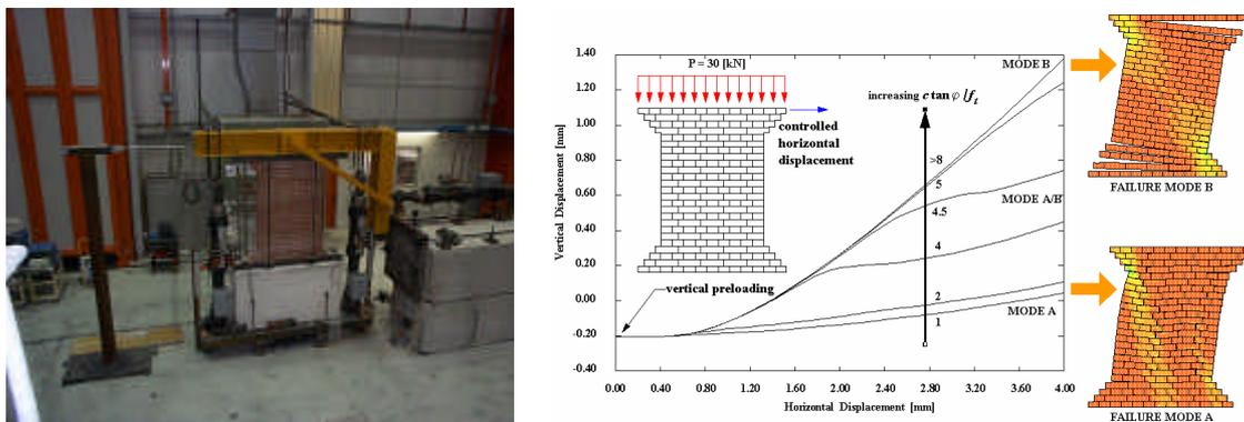
Figure 12: Research on masonry: a) Experimental set-up, b) Numerical simulation
