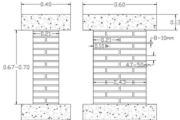
Figure 1: The geometry of specimens
