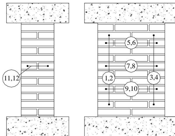
Figure 2 : Location of LVDTs for measuring horizontal and vertical deformations
