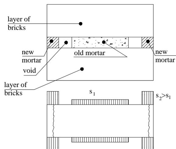
Figure 3 : Compressive stresses on a layer of bricks
