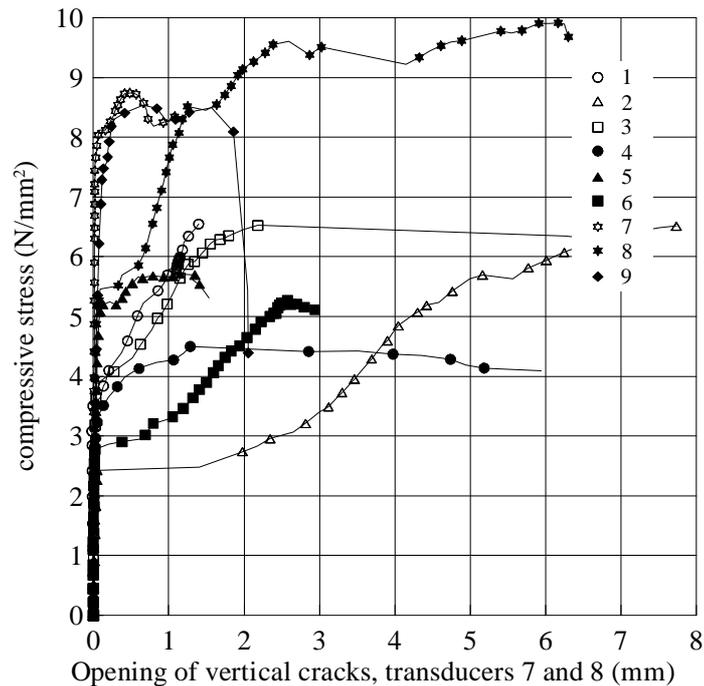
Figure 5 : Compressive stress-opening of vertical cracks curves for prisms 1 to 9
