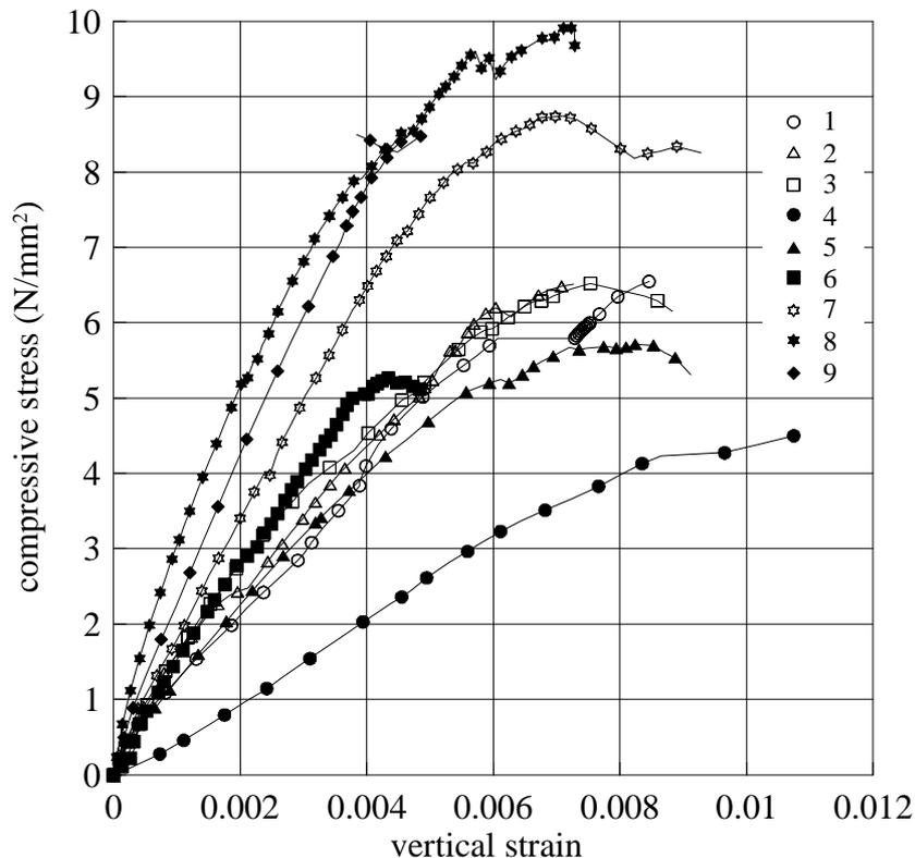
Figure 4 : Stress-strain diagrams for prisms 1 to 9
