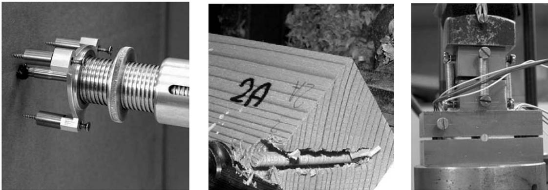
Figure 7 : Drilling machine for extracting a wooden core (left), detail of a drilled core (centre), and testing grips with an inserted oriented core (right).
