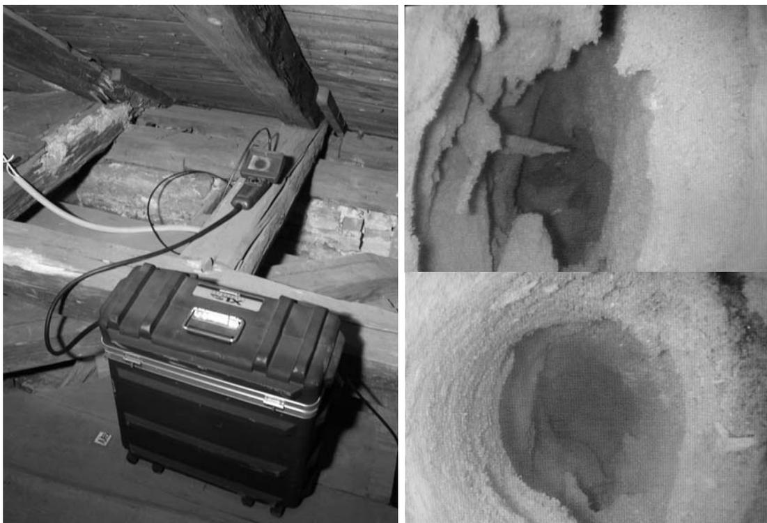
Figure 4 : Videoscapy test arrangement (left), wood decayed by fungi (upper right) and by long horn beetle (lower right)
