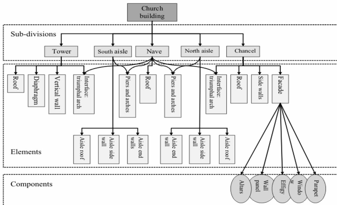
Figure 4 : Typical disassembly for a church
