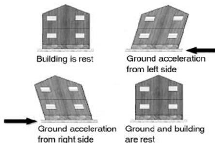
Figure 3: Circular behaviour of timber structures during earthquake (ATC/SEAOC)
