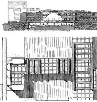
Figure 8 : Zincirli, lower palace wall with wooden grid (Naumann, 1985)
