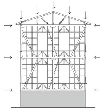
Figure 17 : The load dissipation in a traditional timber framed building (Dışkaya)
