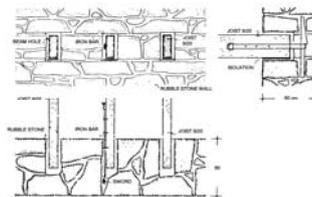
Figure 15 : Tying wooden floor joists to the masonry structure with metal laths (Eldem)
