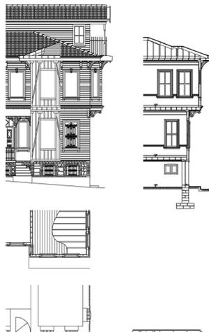
Figure 19 : 19<sup>th</sup> century traditional timber house system detail (Dışkaya)
