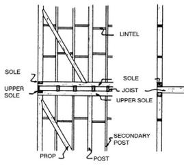
Figure 16 : Timber-framed structure with double sole on both sides (Eldem)
