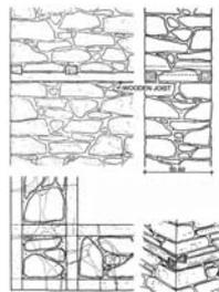
Figure 14 : Rubble Stone wall with wooden joists (Eldem)
