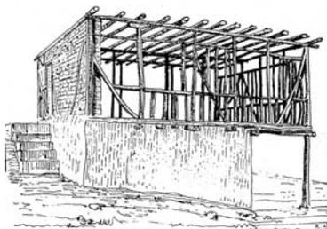
Figure 10 : An infilled wooden structure under construction in Boğazköy in 1957 (Naumann, 1985)
