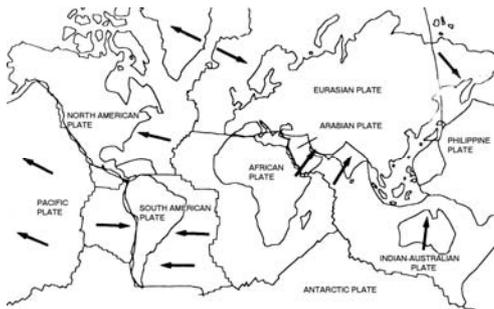
Figure 1: The world's earthquake plates and their movement directions (Celep, Kumbasar, 2004)
