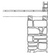
Figure 13 : Timber-Framed Structure Setting on Masonry Foundation (Çobancaoğlu, 1998)
