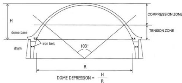
Figure 7 : Typical dome section showing compression and tension zones, and iron belts.
