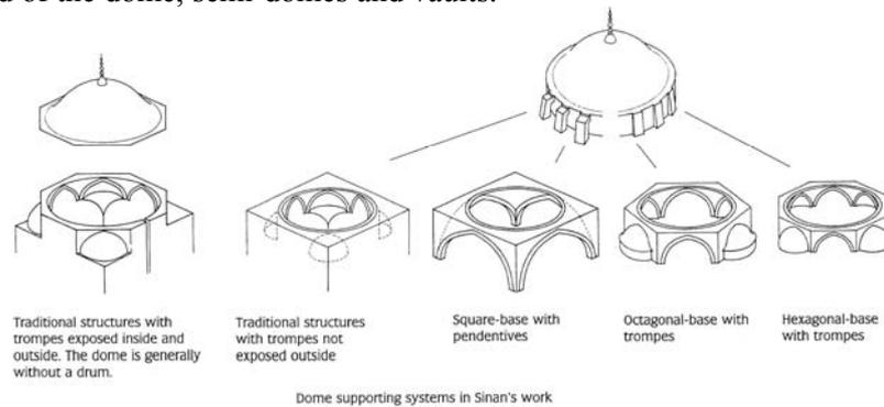
Figure 6 : Dome supporting systems in Sinan's works
