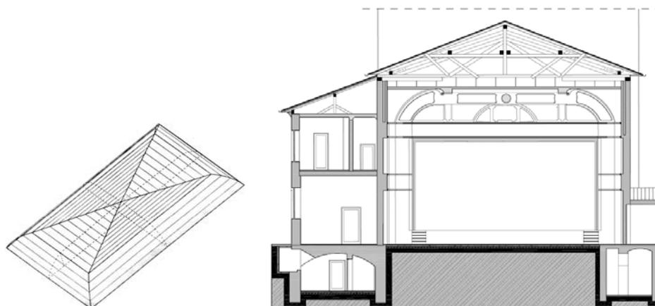
Figure 3 : Mirror vault over the public hall – 3D sketch and cross-section
