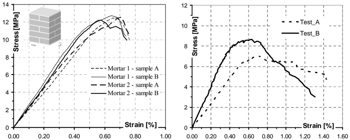
Figure 3 : Stress-strain response under concentric loading for solid clay brickwork: a) 60x120x240 mm bricks, 10mm thick mortar joints – 5 courses; b) 75x140x260 mm bricks, 20mm thick mortar joints – 3 courses.
