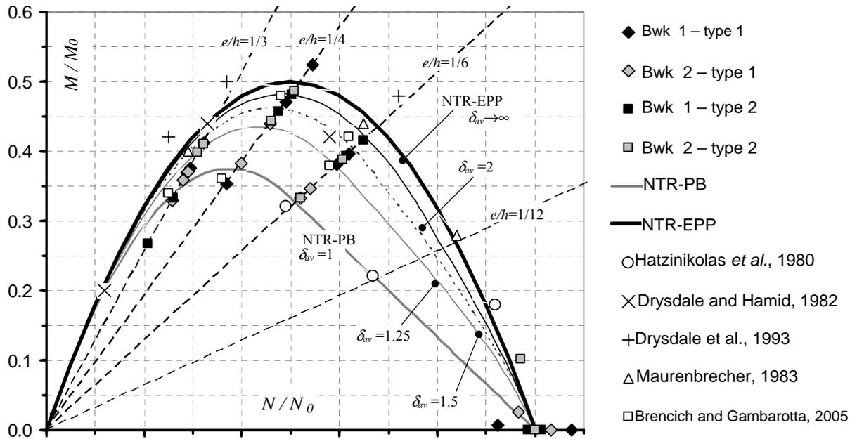
Figure 4 : Limit domains of the NTR-models: exp. data, homogeneous NTR-EPP models with different ductility.
