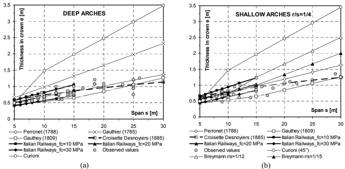
Figure 1 : Thickness in crown vs. span for a) deep and b) shallow (rise/span = 1/4) arches. N-W Italy Dep.ts
