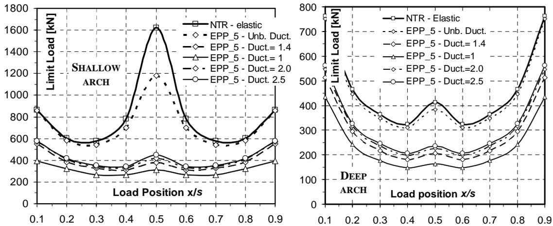
Figure 9 : Limit load vs. load position for the prototype a) shallow; b) deep arches.
