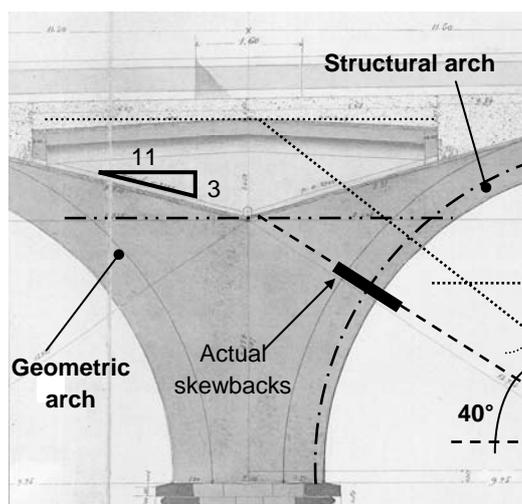
Figure 5 : *Verde viaduct*: section on the pier. Internal spandrels over the backfill.
