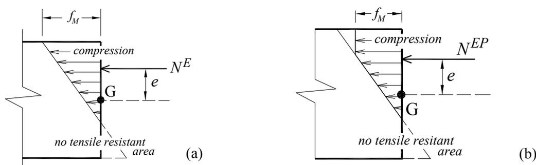
Figure 2 : (a) NTR – Perf. Brittle and (b) NTR-El. Perf. Plastic with limited Available Ductility models for masonry.
