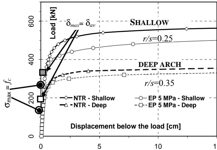
Figure 8 : Load-displacement curves of the prototype arches.
