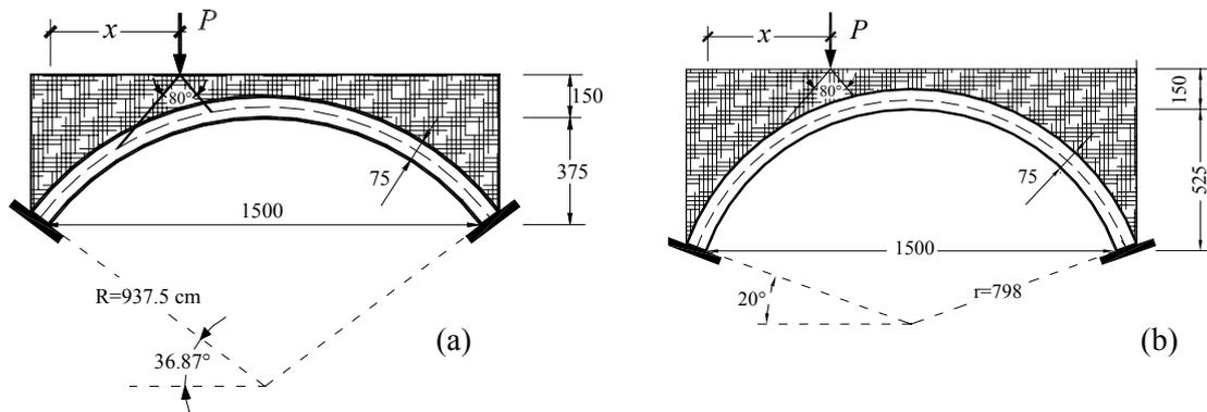
Figure 7 : Prototype arches: (a) shallow ; (b) deep arch.
