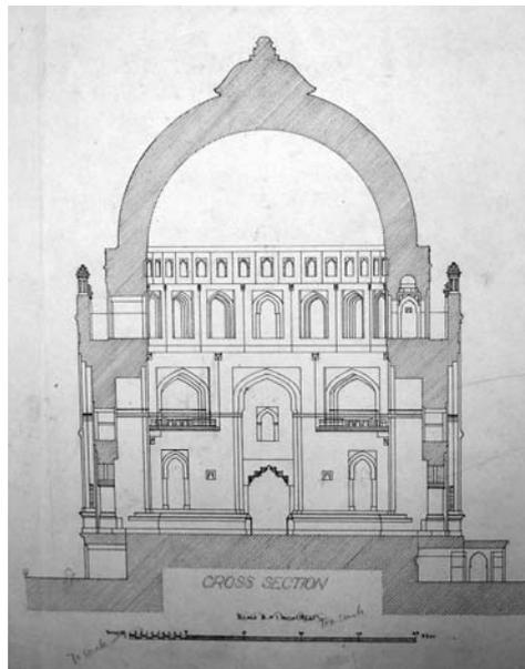
Figure 6 : Section of Bada Gumbad (ASI archives, undated) – an inaccurate drawing that shows hemispherical profile of the dome contrary to ground realities
