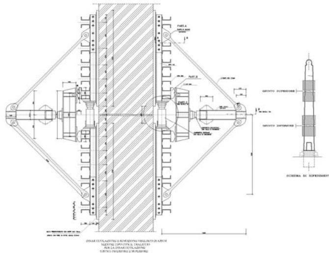
Figure 4 : Axum stelae in Rome, disjuncting operation
