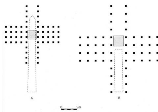
Figure 2 : Plans of the provisional structure for the raising of Vatican's obelisk (A) and of San Giovanni in Laterano one (B), elaborated by M.G. D'Amelio
