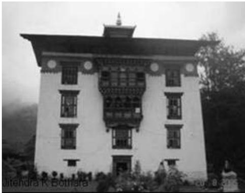
A rammed earth building with trapezoidal wall section (also note wider base, small windows).
