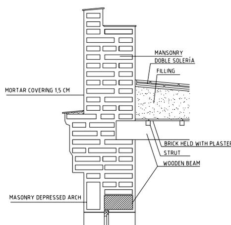
Figure 4 : Constructive section of cornice from Alameda de Hércules st. 45 (Seville)
