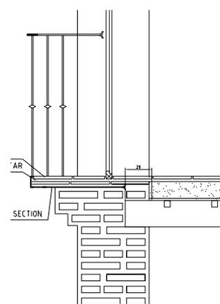
Figure 5 : Constructive section of balcony from Feria st. 97 (Seville)
