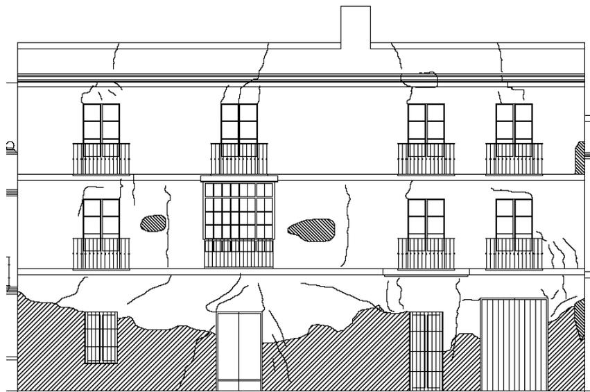
Figure 7 : Drawing of damages. Caballerizas st. 10-12 (Seville)
