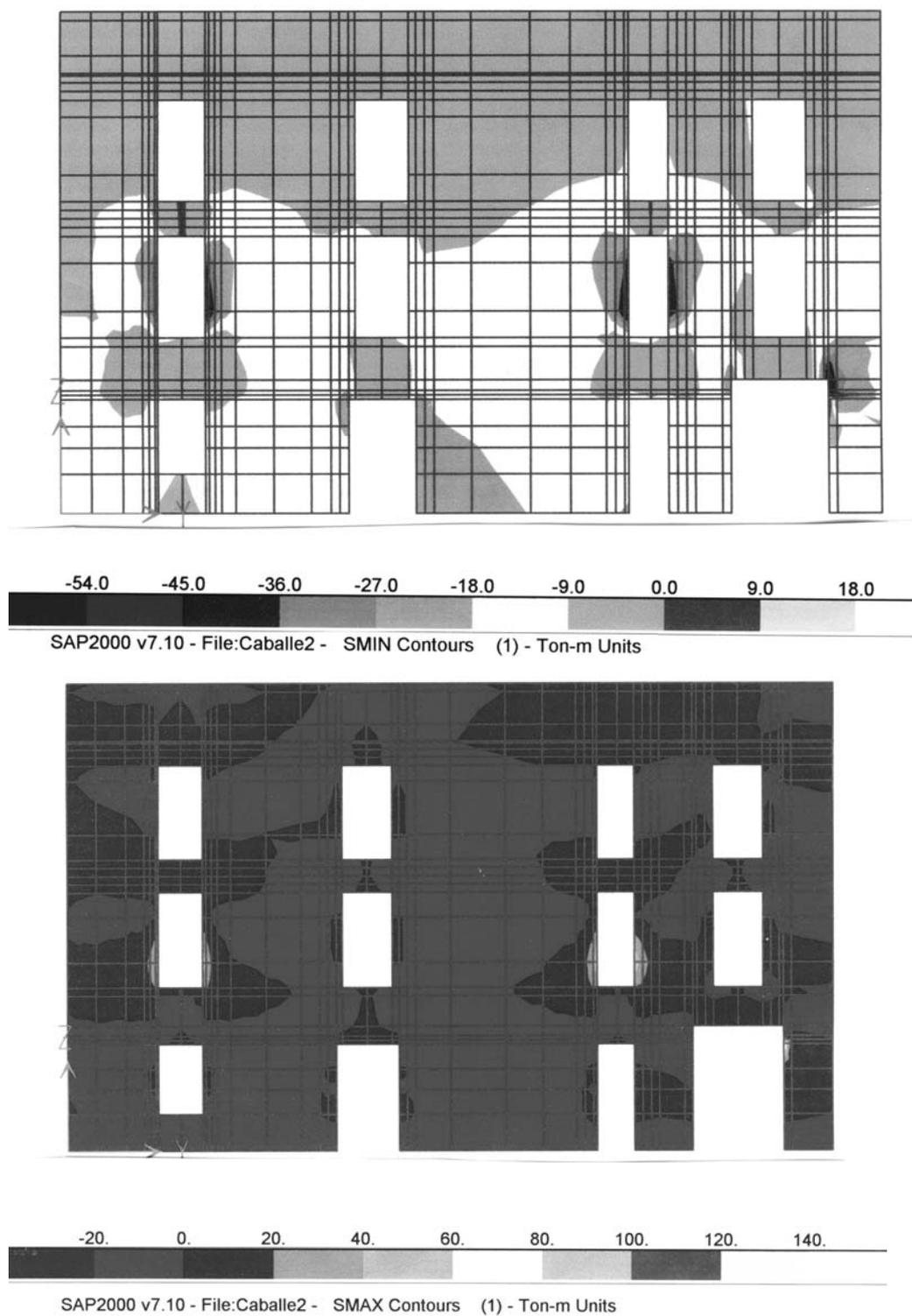
Figure 10 : Diagram of maximum tension (Tractions). Hypotheses 1. Caballerizas st. 10-12 (Seville)
