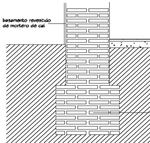
Figure 2 : Generic constructive section of foundations from buildings which belongs to Domestic Sevillian Architecture between 18th and 19th centuries
