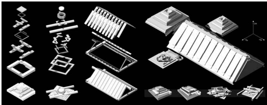
Figure 3 : Solutions for ideal carpentries' reconstructions. Summarizing model of the main ceilings.
