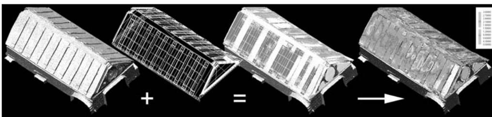
Figure 4 : Inspection procedure. Overlap of the two models and application of “deviation check“.
