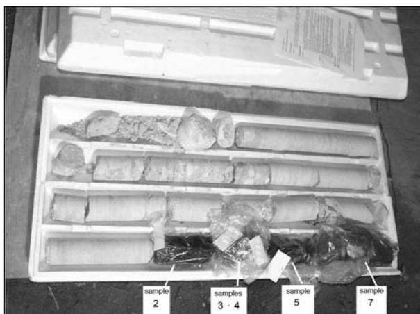
Figure 1 : One of the loggings extracted from building A. As evident, the stone basement of the belfry rests directly on the wooden poles foundation.
