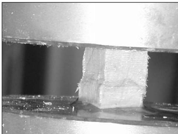
Figure 8 : Buckling of a specimen under load
