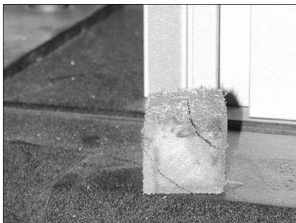
Figure 9 : In some specimens some ring shakes arise during the loading phase. The pattern of such kind of cracks lets suppose that they were already present in the material, even if not visible to a naked eye, at the moment of cutting the specimens
