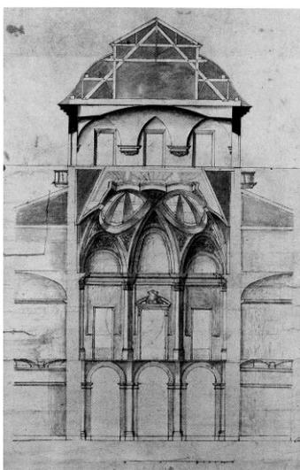
Figure 7 : Castle of Racconigi (CN). Cross-sectional view of the central hall and its roofing. Design project by Guarino Guarini (State Archives of Turin, Az. Savoia-Carignano, categ. 95, m. 2).
