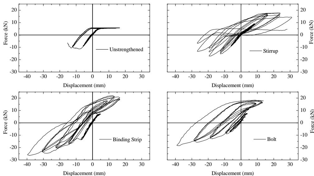
Figure 6 : Force-displacement response for the cyclic loading (rafter compression level of 1.4 MPa).
