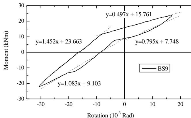
Figure 9 : Final complete cycle for the specimen BS9 (strengthened connection with binding strip).
