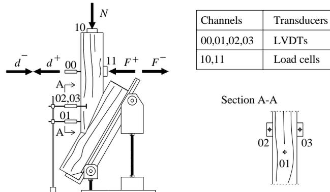
Figure 1 : Testing apparatus and instrumentation layout.
