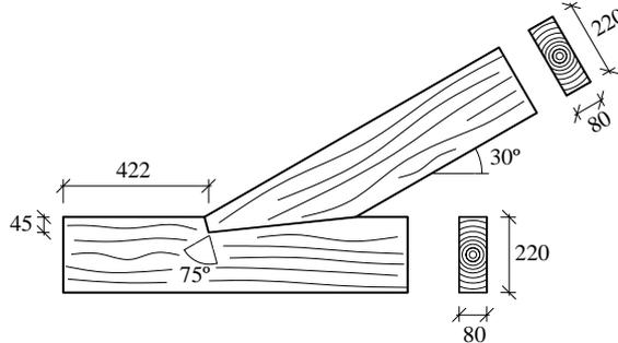
Figure 2 : Connections geometry (dimensions in millimeters).
