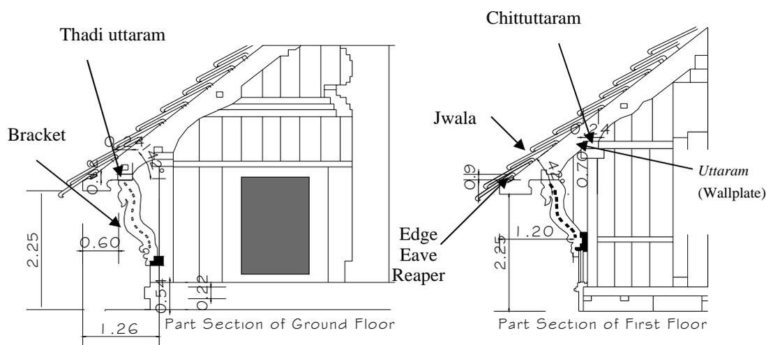
Figure 3 : Part sections of a typical palace superstructure.
