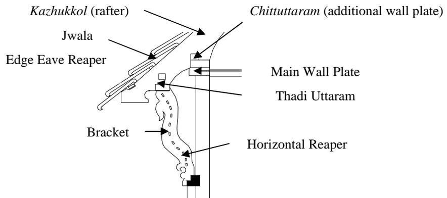
Figure 2 : Details at the end of the rafter.
