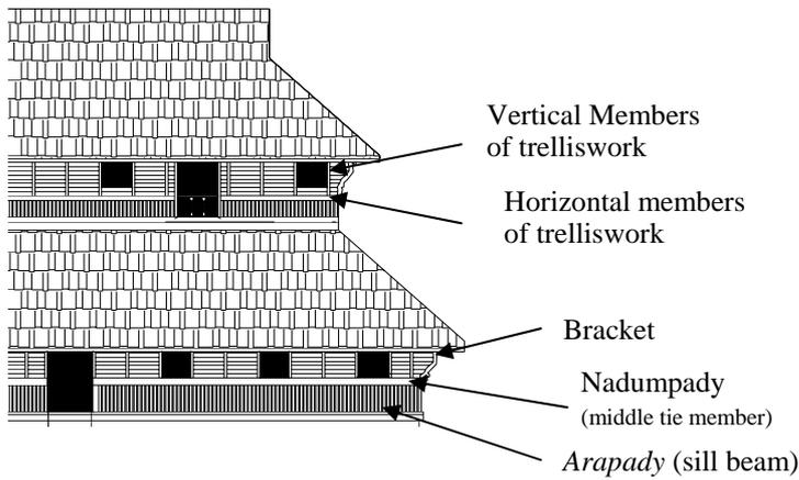
Figure 1 : Parts of a typical palace.
