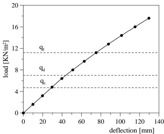
Figure 10 : Load-deflection for strengthened floor 2.
