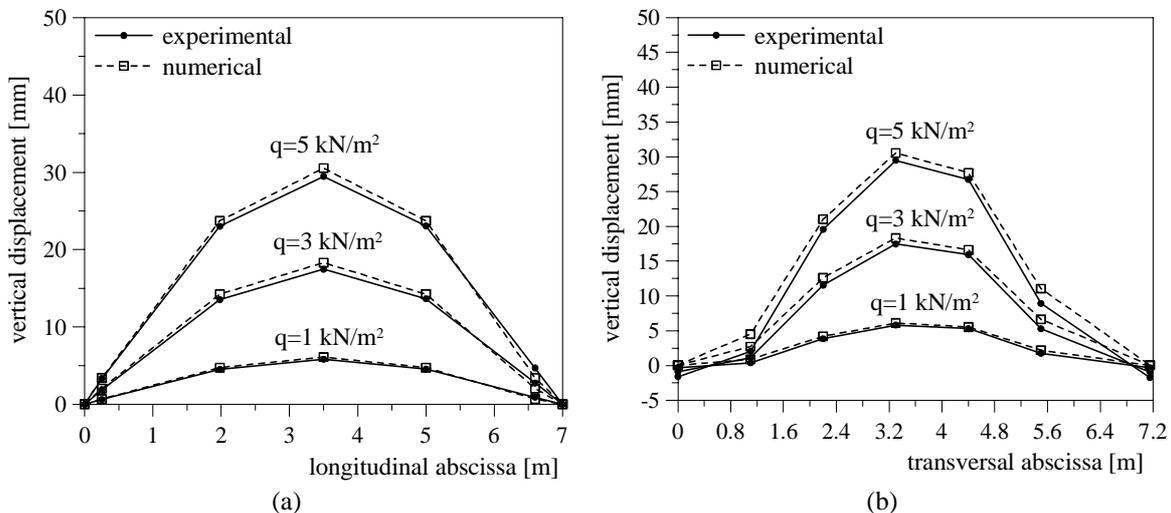
Figure 8 : Displacements of the strengthened floor 2: (a) longitudinal direction, (b) transversal direction.
