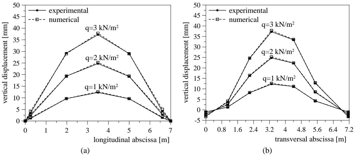
Figure 7 : Vertical displacements of the plain floor 2: (a) longitudinal direction, (b) transversal direction.
