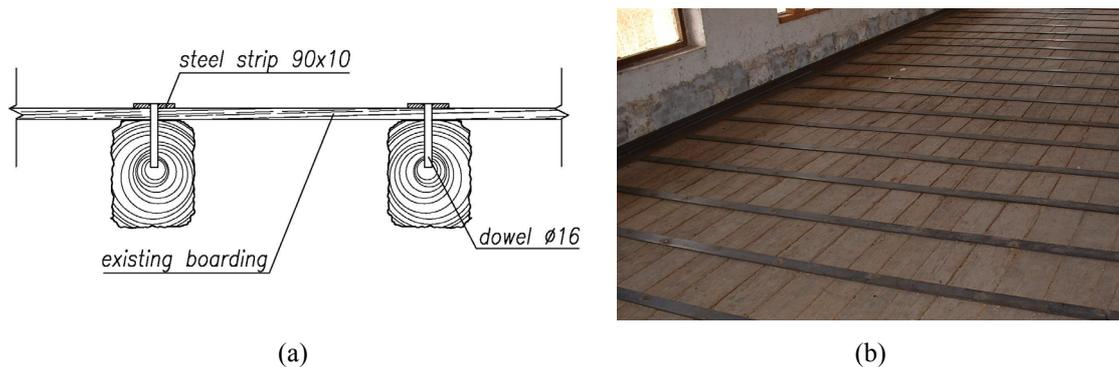
Figure 1 : Strengthening technique: (a) cross section, (b) stiffened floor example.
