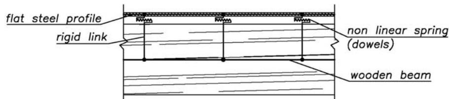
Figure 9 : Modeling of the composite system.
