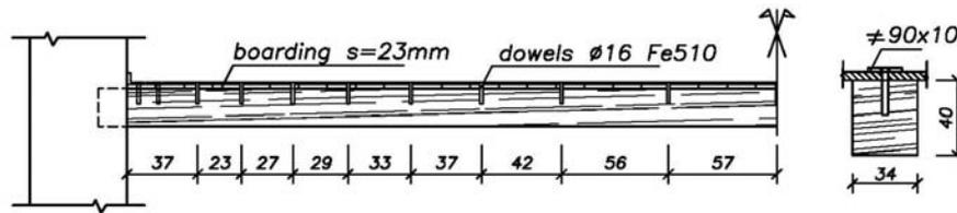
Figure 6 : Distribution of dowels along half a beam and cross section.
