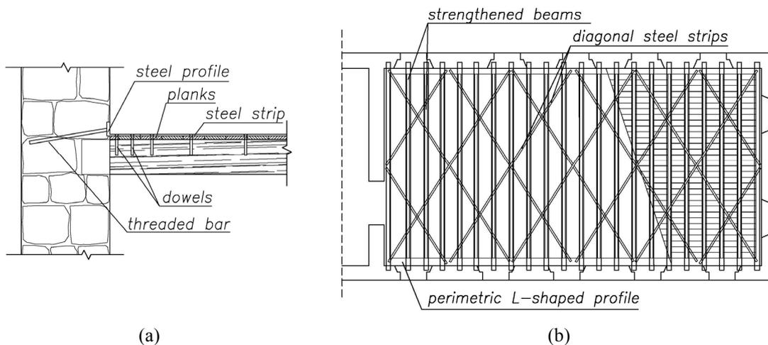
Figure 2 : Details of the complete intervention: (a) floor-wall connection, (b) lattice truss system.
