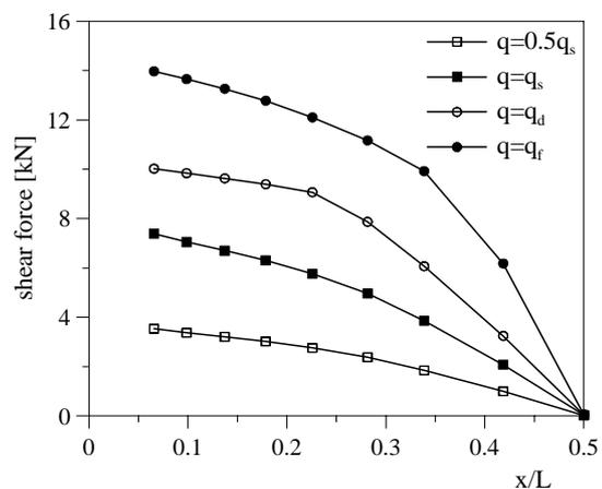
Figure 13 : Shear force on dowels along half span for floor 2.
