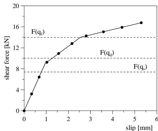
Figure 11 : Load-slip for outer dowels of floor 2.
