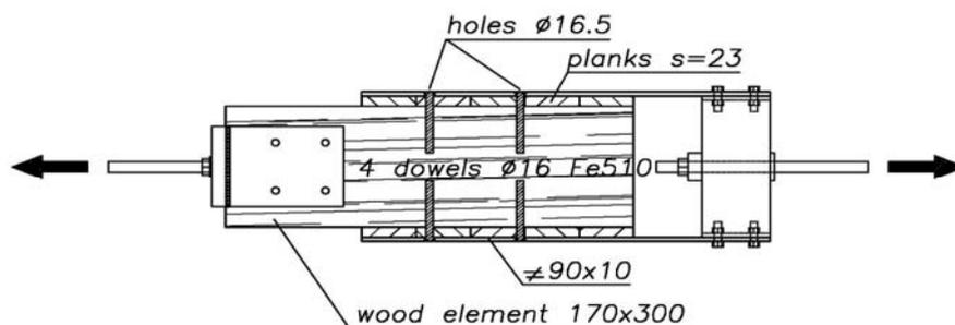
Figure 3 : Specimen for tests on the connection.
