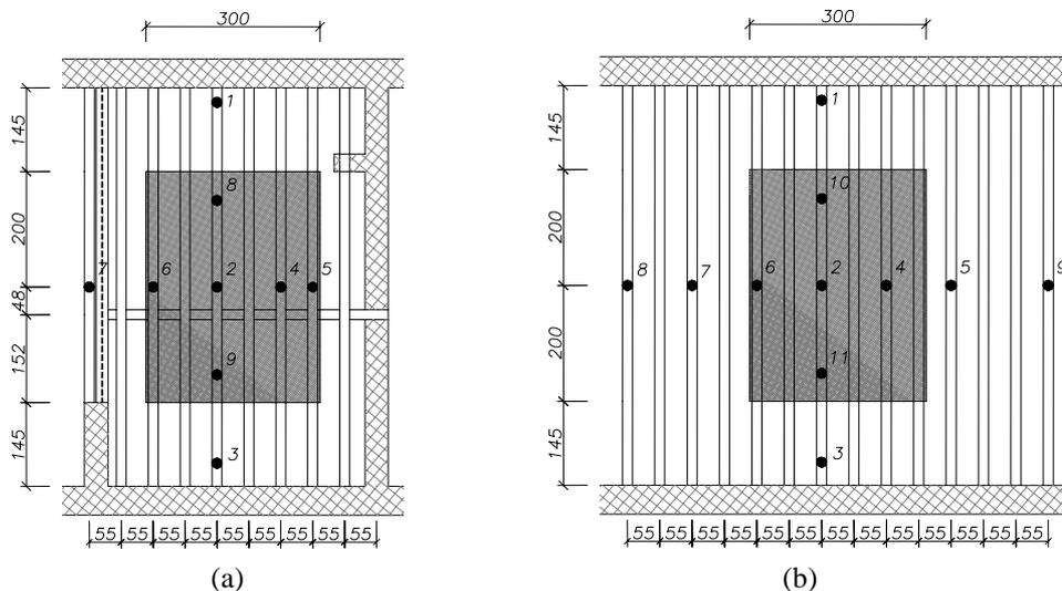
Figure 5 : Loaded portion of the floors and position of the transducers: (a) floor 1, (b) floor 2.
