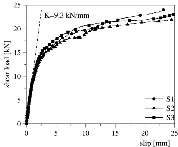
Figure 4 : Results of tests on the connection: load-slip relationship of the single dowel.
