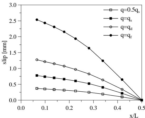
Figure 12 : Steel-wood slip along half span for floor 2.
