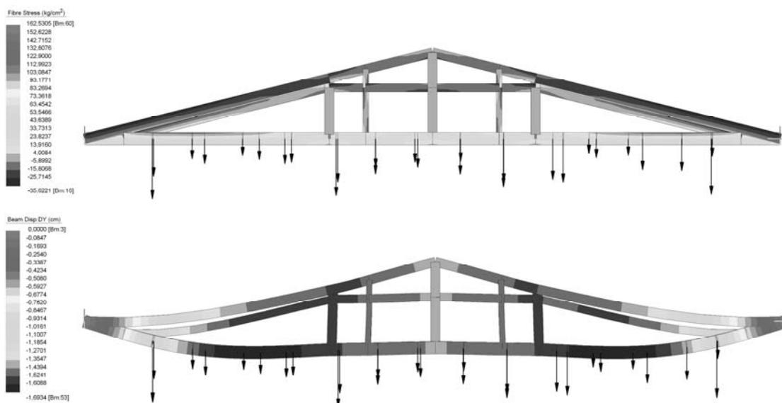
Figure 3 : Numerical model of the 7<sup>th</sup> Graldi's truss. The painted ceiling is suspended from this truss. Structural unit subjected to static loads. Stresses (up). Vertical displacements (down).
