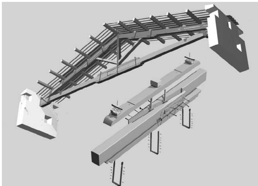
Figure 5 : The vasarian truss; exploded view of the chord.
