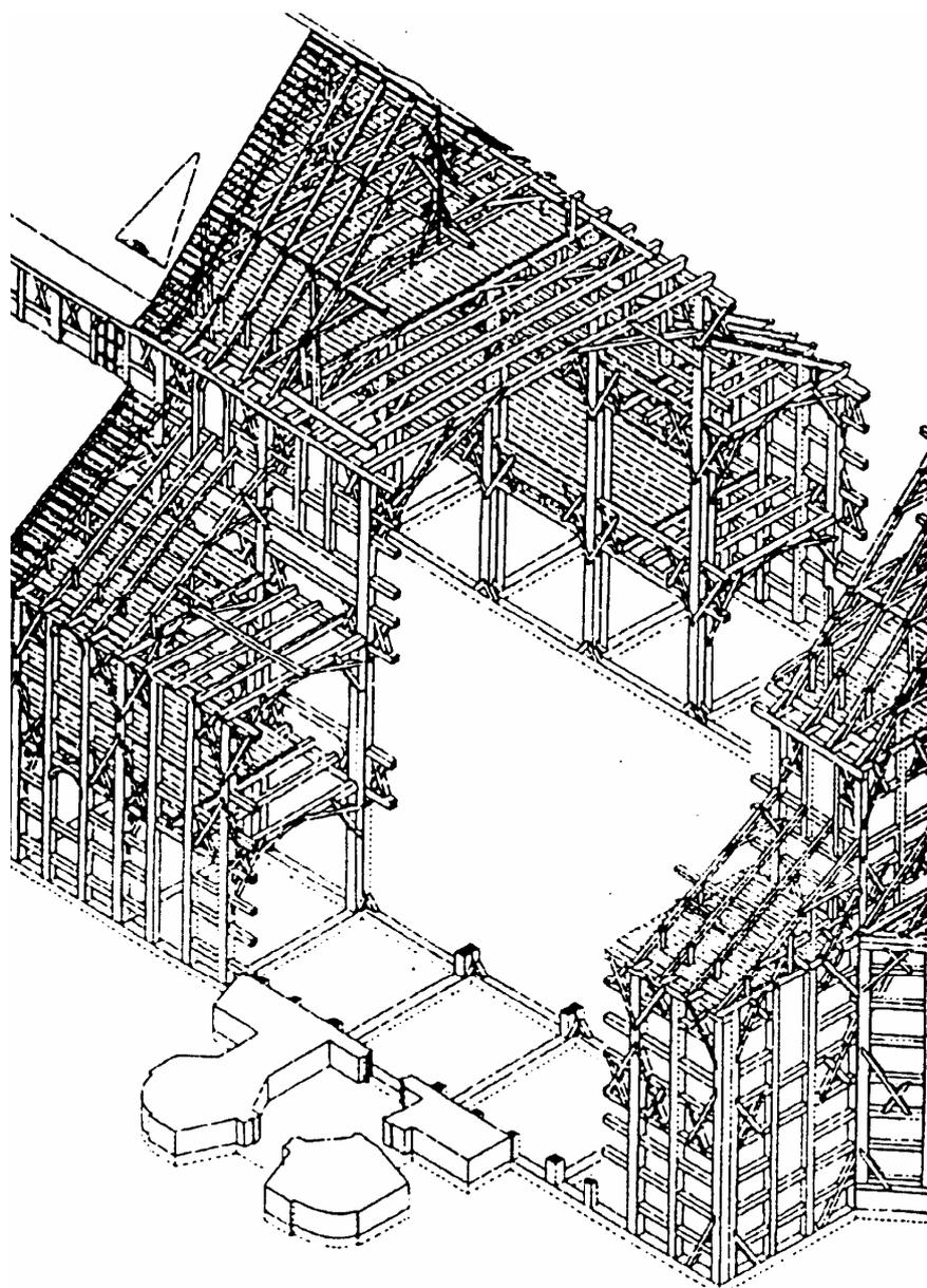
Figure 3 : Axonometric view of the fragment of church skeletal construction from southern side.
