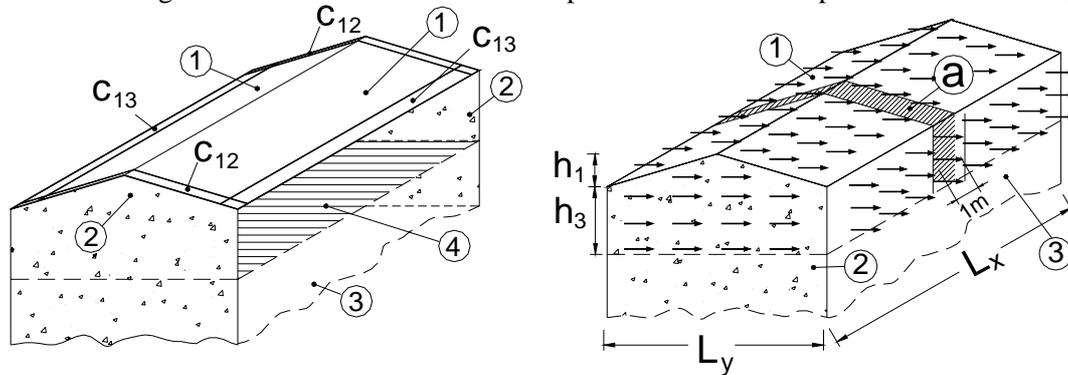
Figure 3 : (a) Structural elements for the wooden roof strengthening; (b) seismic action distribution.
