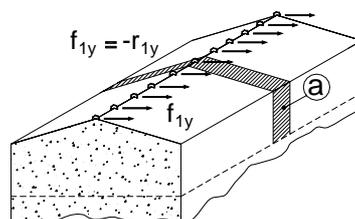
Figure 5 : Box-structure undergoing horizontal ridge loads.
