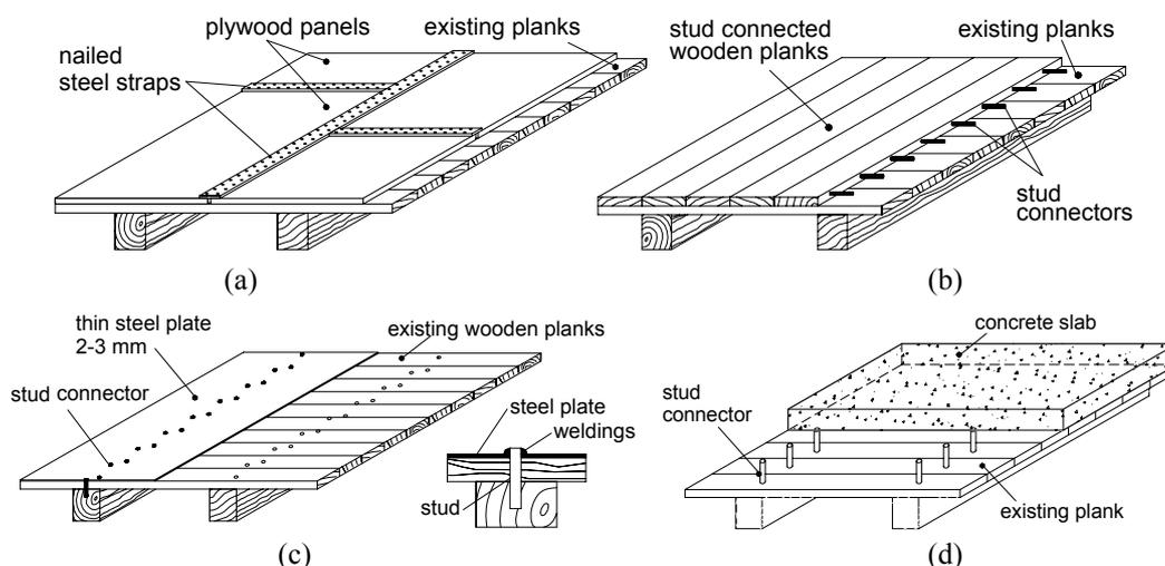
Figure 2 : Wooden floor in plane shear strengthening by means of (a) plywood panels; (b) stud connected wooden planks; (c) thin steel welded plates; (d) thin concrete slab.
