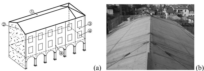
Figure 7 : Palazzo Calini ai Fiumi: (a) simplified scheme of the structure; (b) antiseismic wooden roof.
