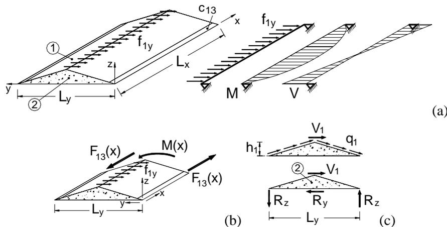
Figure 6 : Simplified schemes for the evaluation of the force distribution in the box structure.
