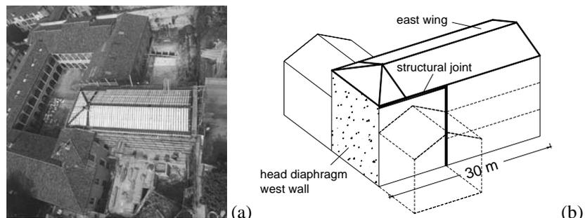
Figure 8 : Santa Chiara: (a) aerial view; (b) simplified scheme of the structure.
