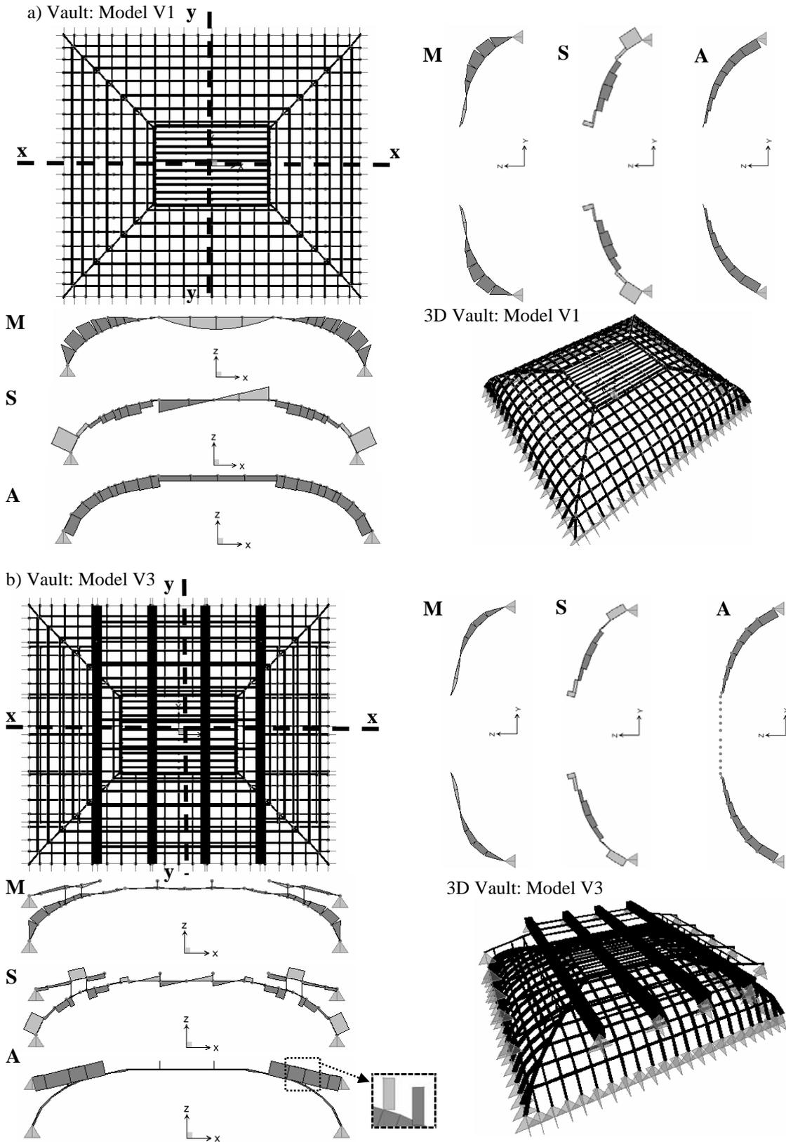
Figure 3 : Internal forces distribution in the vault elements.
