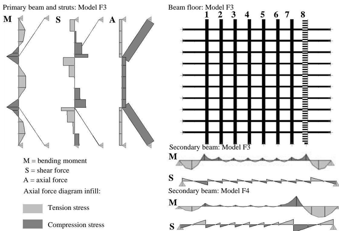
Figure 2 : Internal forces distribution in the floor beams
