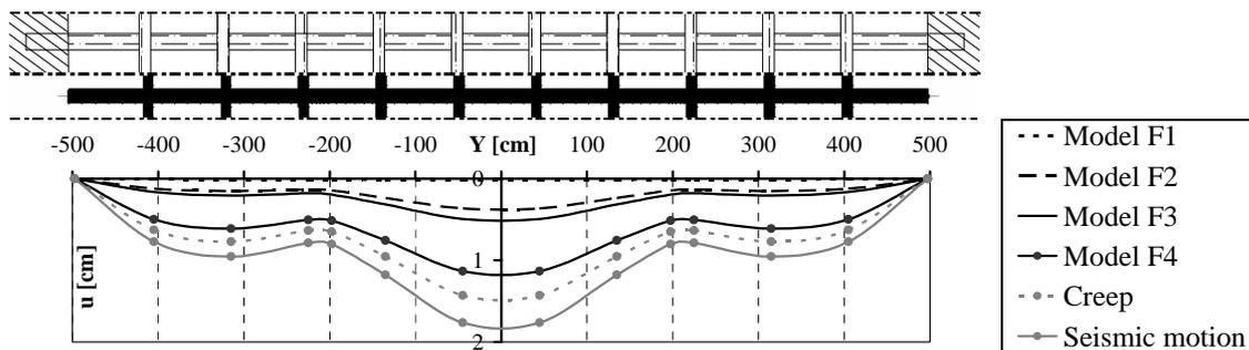
Figure 4 : Vertical displacements of the floor beam n. 7 for each examined structural model.
