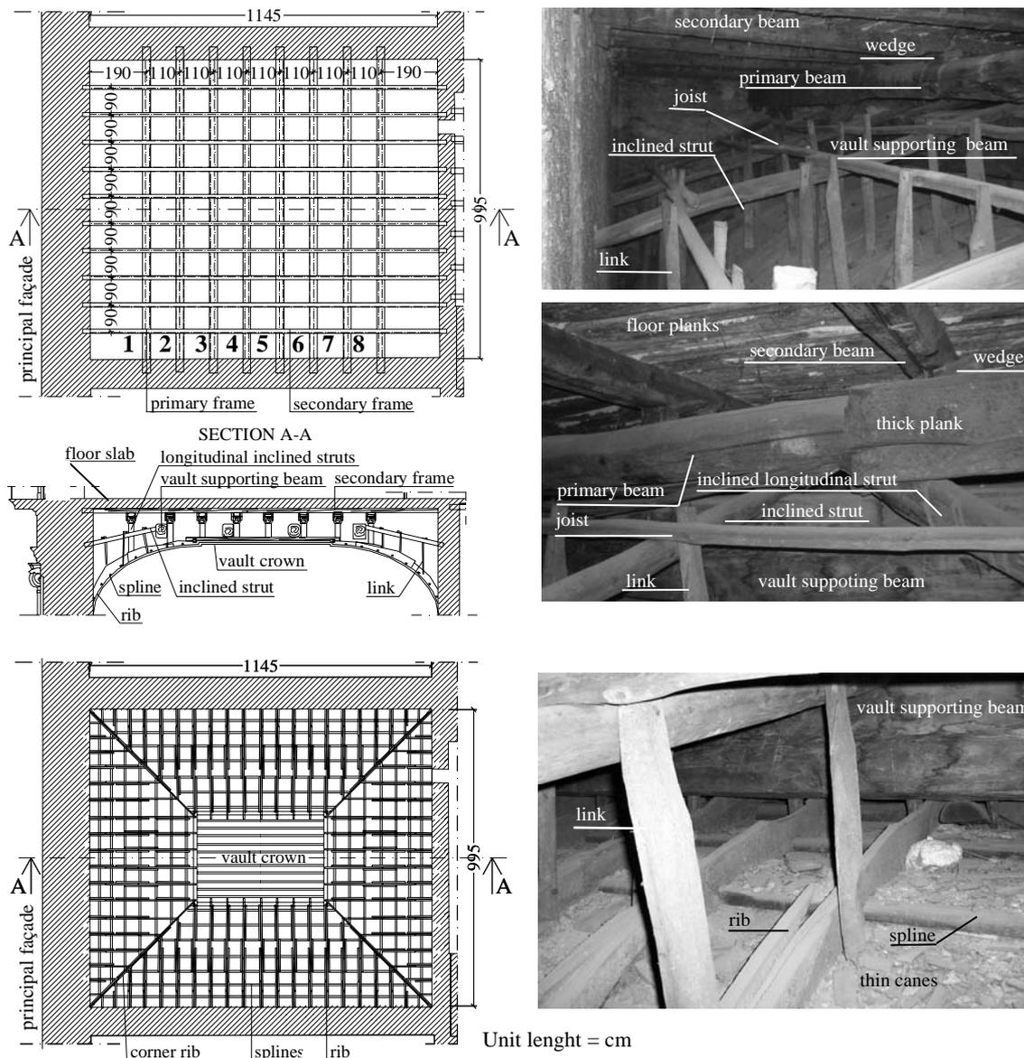
Figure 1 : The second Anteroom roofing structures.
