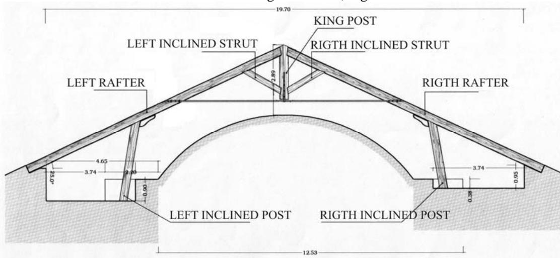
Figure 3 : Survey of the truss
