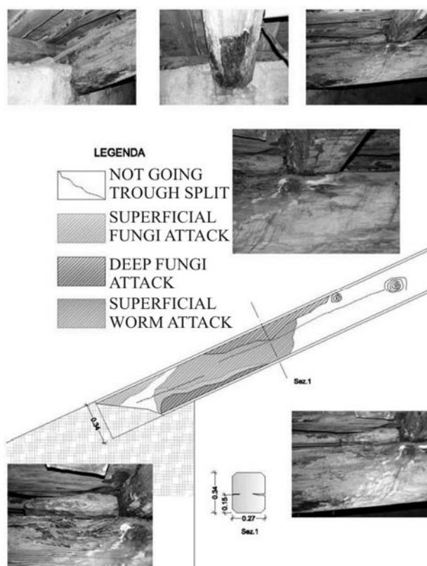
Figure 4 : Chart with the map of decay, for the left rafter.
