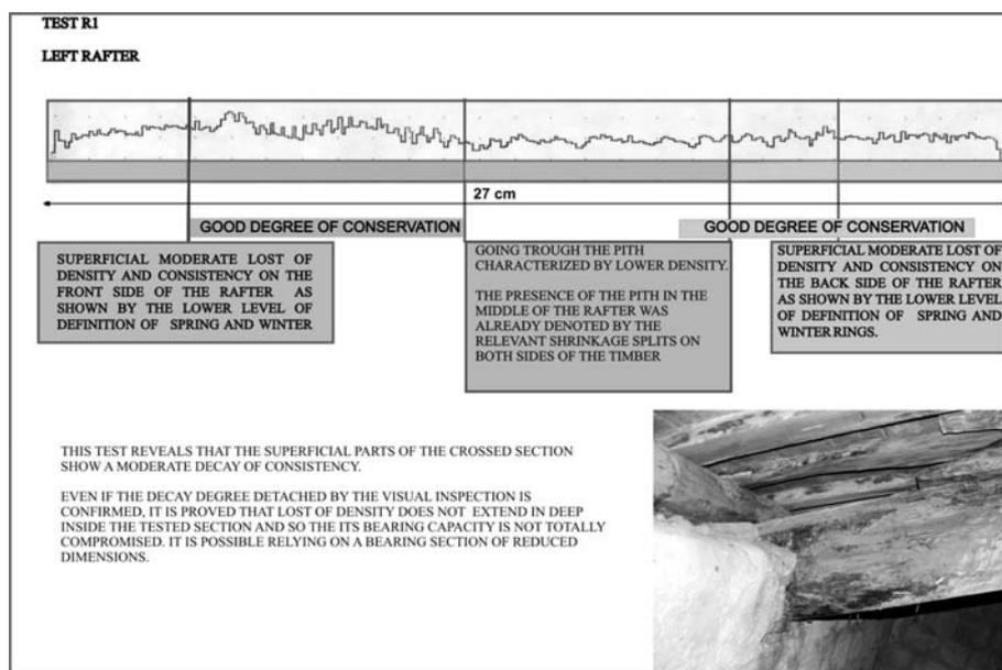
Figure 5 : Resistographic chart of the left rafter.
