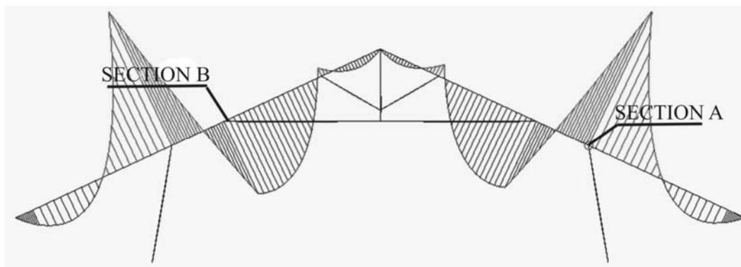
Figure 7 : Bending moments diagram.
