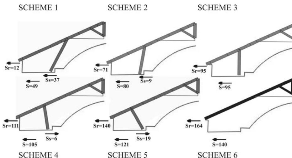
Figure 8 : Different calculated schemes with values of the thrusts.
