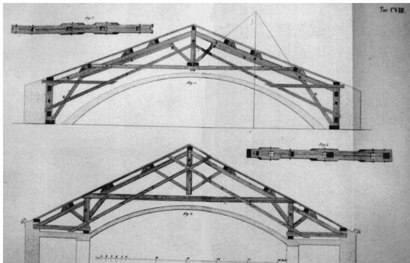
Figure 2 : Drawing of the Pantheon trusses
