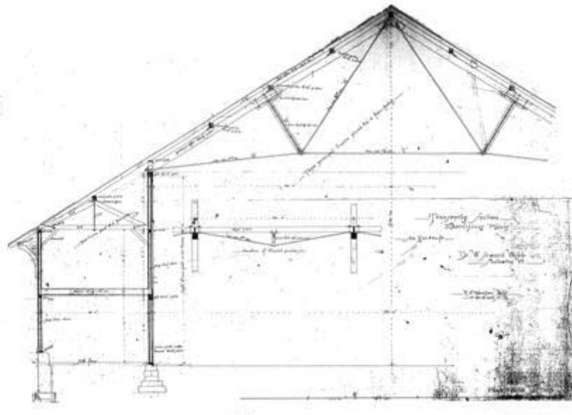
Figure 4 : A portion of the transverse section drawn by Robertson and illustrating the principal truss (Collection, Shelburne Farms Archive).
