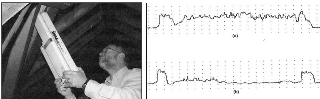
Figure 3: Resistance drilling was done to characterize the extent of deterioration in decayed frame members, left. At right, the top graph depicts sound timber (a), while the graph at bottom depicts timber with internal deterioration (Anthony 2006).
